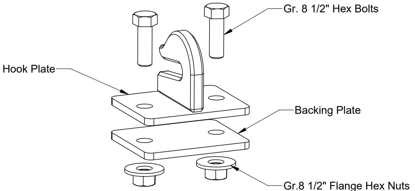
1. Place hook plates in desired locations. Use as templates to mark hole locations.
