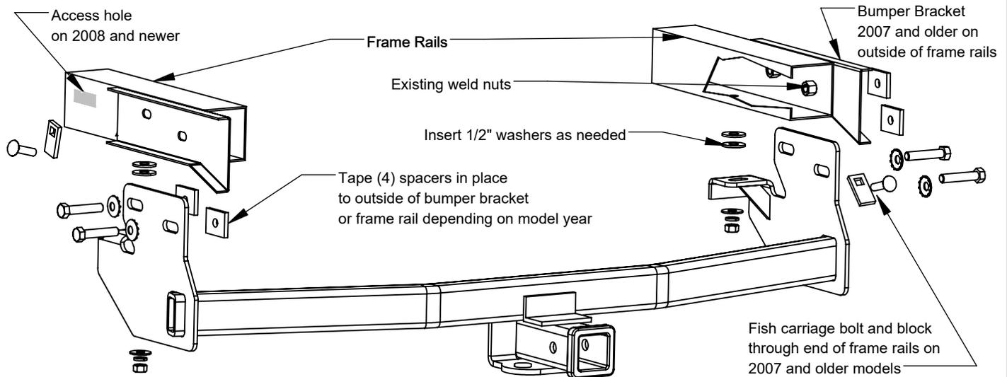
1. Remove the (4) bolts (2 per side) on the vertical sides of the frame rails that attach the bumper brackets to the frame, and return to owner. **Note:** On 2007 and older models the bumper brackets are on the outside of the frame rails. On 2008 and newer models the bumper brackets are inside the frame rails.
