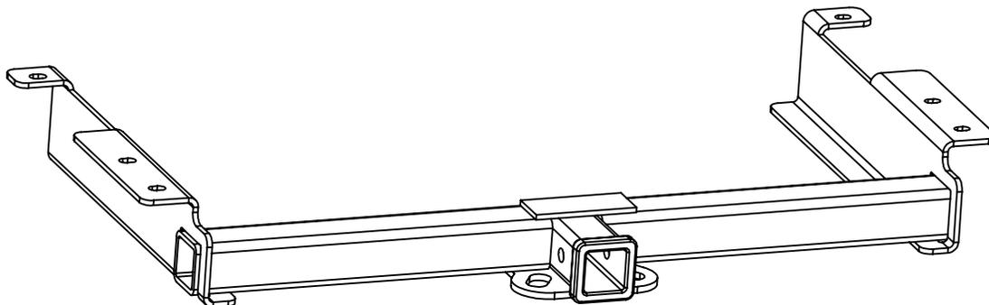
1. Assemble the (6) 1/2-13 x 1-3/4" carriage bolts and (6) 1/4 x 1-1/2 x 2" block plates.
