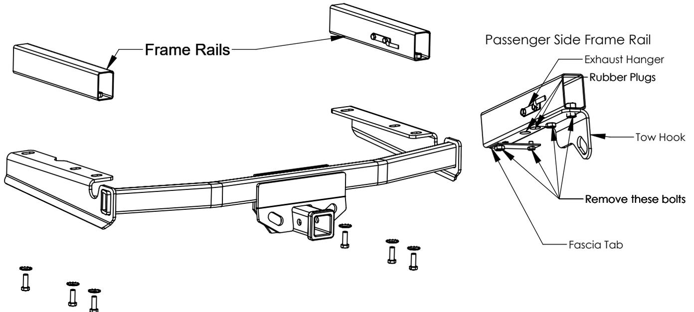
1. Remove the (5) fasteners securing the driver side underbody appearance panel. Pull the appearance panel downward to release it from the two studs holding the panel in place. Return the appearance panel and fasteners to the vehicle owner. Remove the two plastic push pins securing the rear bumper fascia tabs, using a flat blade screw driver to pry the center of the pins downward, bend fascia tabs down.
