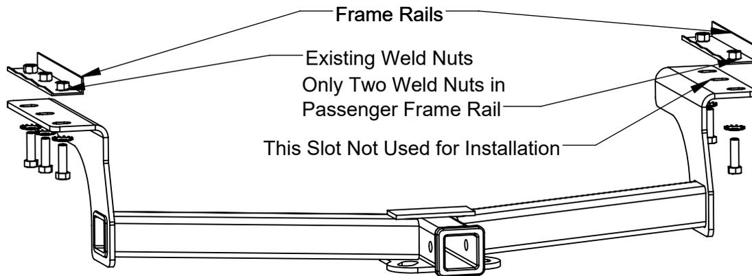
1. Remove appearance panel and tow hook from driver's side frame rail and return to owner.
