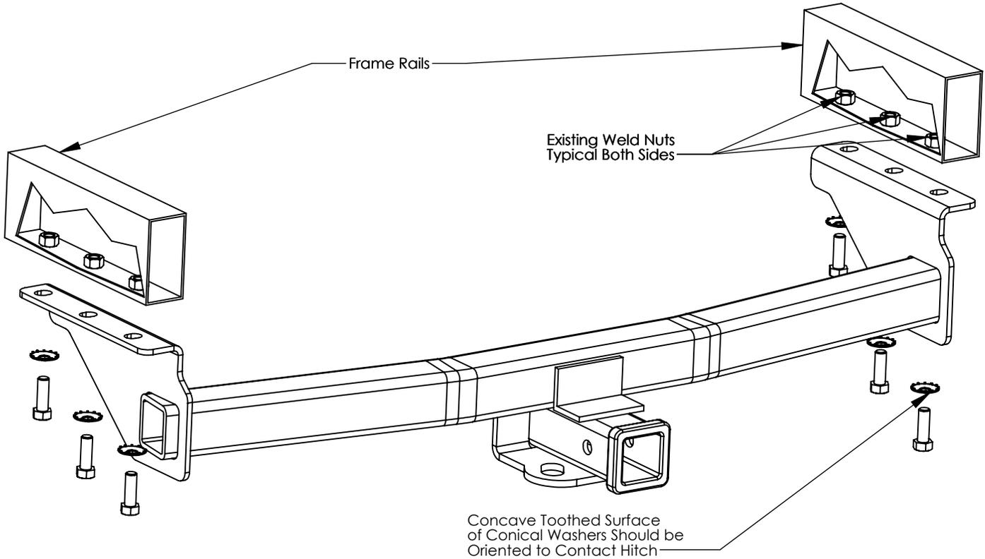
1. Raise the hitch into position and insert the six M12 hex bolts and conical washers into the six existing weld nuts in the frame rails.
