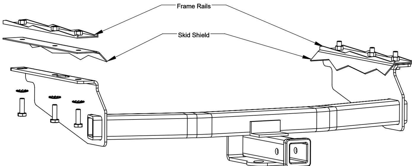
1. If the vehicle is equipped with a fuel tank skid shield, remove and discard the six M12 fasteners. The skid shield will be sandwiched between the frame rails and the hitch.
