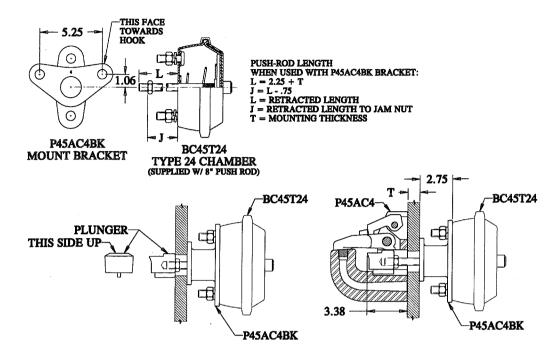
3b. When using any other air chamber mounting structure determine the cut length as follows:
