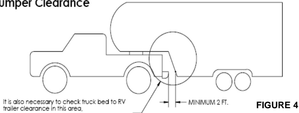
4. A minimum clearance between the bumper and trailer (Measured at the same height) of 2 ft. is recommended (Figure 4).
