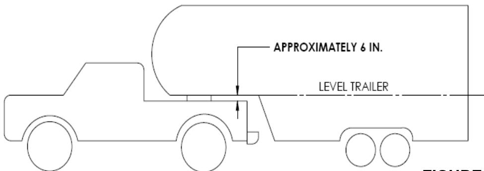
5. The height of the hitch and pin box should be adjusted so the trailer is approximately level as it is towed. Allow approximately 6 in. clearance between the top of the bedside and the underside of the front of the trailer for pitch and yaw of the trailer (Figure 5).
