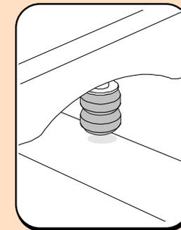
Do not exceed vehicle manufacturer's recommended axle weight rating. Check for AEON® interference with vehicle components - Under load AEON® will "expand" in diameter.
