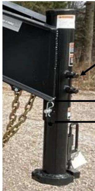
Set bolts are to face front of trailer toward tow vehicle. Set bolts are to torqued at 90 ft lbs.
