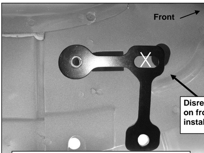
(Fig 3) Front Bracket Spacer on driver side
