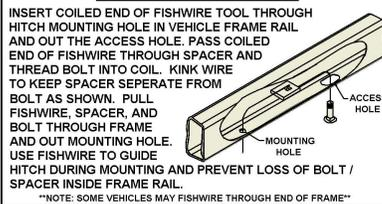
INSERT COILED END OF FISHWIRE TOOL THROUGH HITCH MOUNTING HOLE IN VEHICLE FRAME RAIL AND OUT THE ACCESS HOLE. PASS COILED END OF FISHWIRE THROUGH SPACER AND THREAD BOLT INTO COIL. KINK WIRE TO KEEP SPACER SEPARATE FROM BOLT AS SHOWN. PULL FISHWIRE, SPACER, AND BOLT THROUGH FRAME AND OUT MOUNTING HOLE. USE FISHWIRE TO GUIDE HITCH DURING MOUNTING AND PREVENT LOSS OF BOLT / SPACER INSIDE FRAME RAIL.
