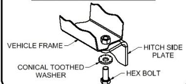
**PERIODICALLY CHECK THIS GOOSENECK HITCH TO ENSURE THAT ALL FASTENERS ARE TIGHT AND THAT ALL STRUCTURAL COMPONENTS ARE SOUND.**
