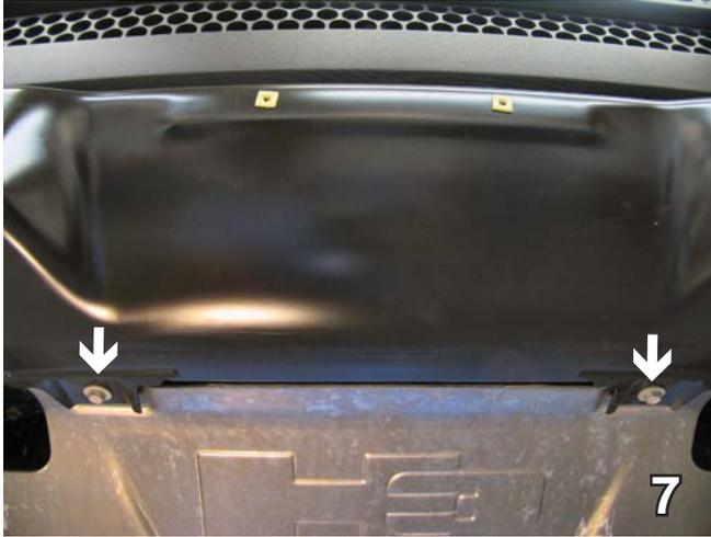
7. On the bottom side of the lower front fascia, where the belly pan meets the lower front fascia, remove two metric bolts using a 13MM Socket. When the bolts have been removed, set them aside as they will need to be reinstalled.
