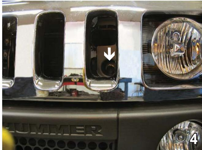
4. Inside the grill, near the headlight assembly remove one metric bolt using a 10MM Socket. This procedure is done on both sides of the vehicle, the driver's side is shown.
