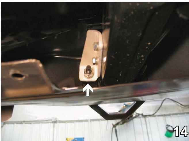
14. Remove the existing bolt, 12MM hex nuts (reference #9 on page 5 of this document) and replace fascias according to the directions on the previous pages. This procedure is done on both sides of the vehicle, the passenger's side is shown.
