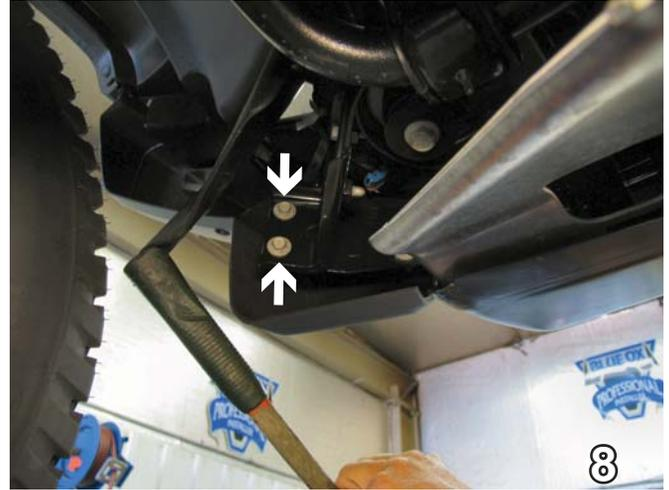
8. Next you will need to pull back, but **DO NOT REMOVE**, the webbing from the underneath side of the lower front fascia and remove 2 metric bolts using a 13MM Socket. Set these bolts aside as they will need to be re-installed. This procedure needs to be done on both sides of the vehicle, the driver's side is shown.
