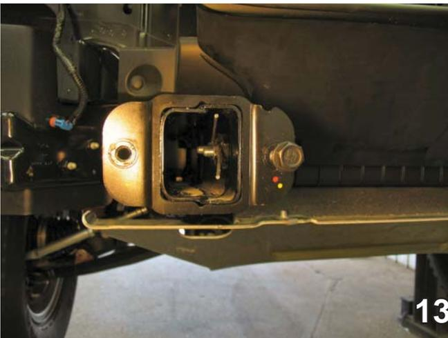
13. Insert the nut plates into the frame rail to align with drilled holes and tighten the 3/8"-16 hex bolts and 3/8" lock washers according to the torque chart on page one of this document. **(BE SURE TO USE LOCTITE RED.)** This is done on both sides of the vehicle, the passenger's side is shown.
