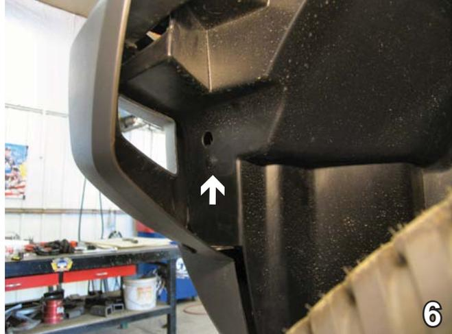
6. On the backside of the lower fascia, remove one push pin from the lower front fascia. Set the push pins aside as they will need to be re-installed. This procedure is done on both sides of the vehicle, the driver's side is shown.
