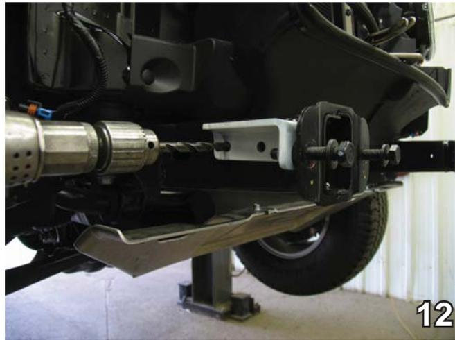
12. Using the baseplate as a template, drill the holes with the 13/32" drill bit, for the baseplate to mount to the frame rail.
