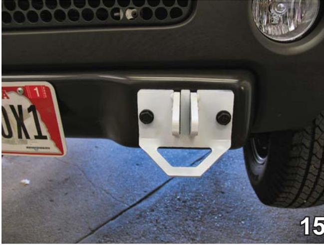
15. Align baseplate with existing holes on front of metal bumper fascia. Tighten existing bolts to go through the bracket. Replace lock washer and hex nut to back side of the fascia, as shown in step #14. This procedure is done on both sides of the vehicle, the driver's side is shown.
