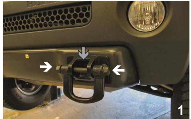
1. Using a 24MM Socket, remove the tow hooks from the front fascia. Set aside and return to customer as these will **NOT** be reinstalled on the vehicle. Some models will have bolts to remove with a T-30 Torx socket. This procedure will need to be done on both sides of the vehicle, the driver's side is shown.
