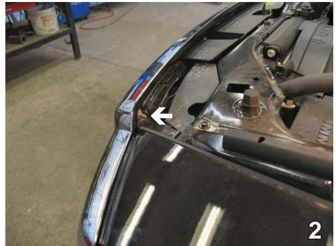
2. The upper and lower front fascias will need to be removed for this baseplate installation. Using a 10MM Socket, remove one metric bolt from behind the upper front fascia. This procedure is done on both sides of the vehicle, the driver's side is shown.
