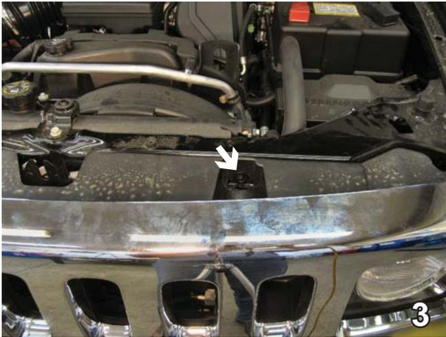
3. On the front side of the upper front fascia, using a 10MM Socket, remove one metric bolt. Set aside as these bolts will need to be re-installed. This procedure is done on both sides of the vehicle, the driver's side is shown.
