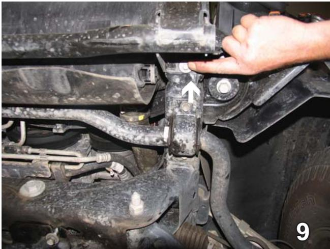
9. **2009 Models:** Using a 10MM socket, remove the metric bolt from the impact bar support. Do this on both sides. Set the bolts aside to be reinstalled after the bracket is attached in step 11.
