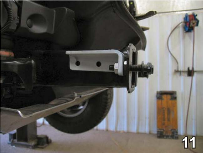
11. Using the existing bolts (Reference #9 on page 5 of this document) insert but do not fully tighten the bracket so that it sits up next to the frame rail.
