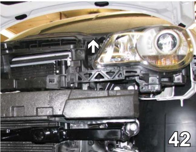
42. Put the headlight brackets and the headlights back in and reconnect.
