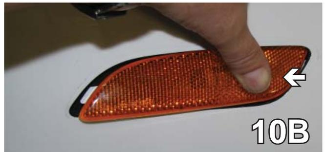
10. On the back of the side marker lights, press the clip down to release. On the front, slide the light in and back, the front comes out. Pull the light out, then push the light in the opening and out the back. On the back side of the fascia on the driver's side only, detach the marker light from the clip. Unplug the running lights. Pull fascia corners out to the side, pull fascia forward to remove. Set fascia aside carryover to reinstall later.
