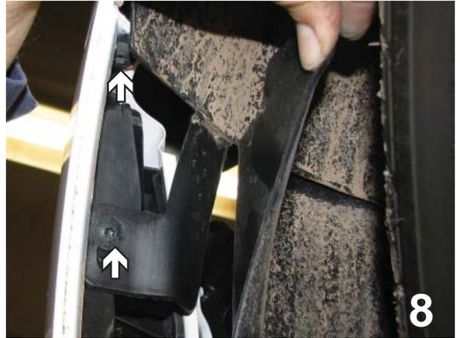
8. Pull the wheel well cover back and remove two T-25 Torx screws. Set screws aside to reinstall later. Also pull the slide bar back until it clicks to release the clips holding the fascia. Do this on both sides.
