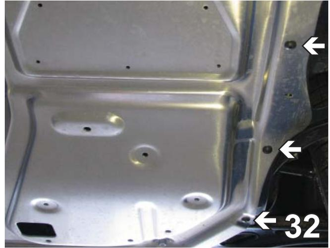
32. If the two bottom holes of step 30 do not line up, it may be necessary to separate the belly pan from fender well plastic using the T-25 Torx to remove the three torx bolts on both sides. Pull wheel well plastic back to ream existing holes.
