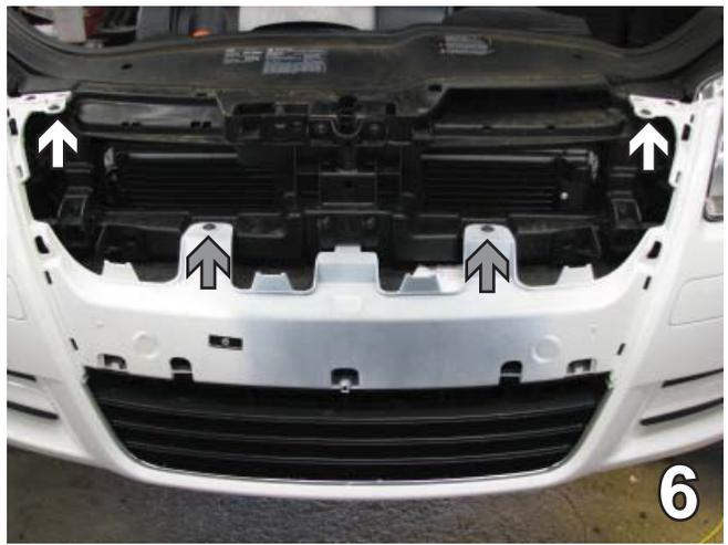
6. Just behind grille, remove two T-25 Torx bolts at the top (white arrows). And two T-30 Torx bolts in the center (gray arrows). Set bolts aside to reinstall later.
