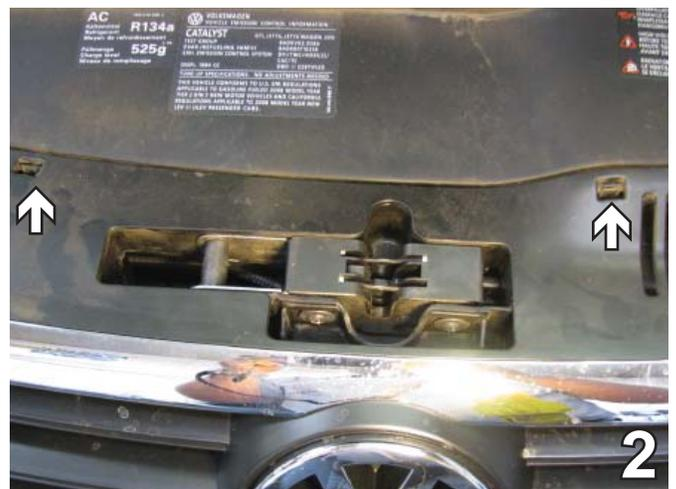
2. Pull back on the two clips in order to remove the plastic. Set plastic aside for later reinstallation.
