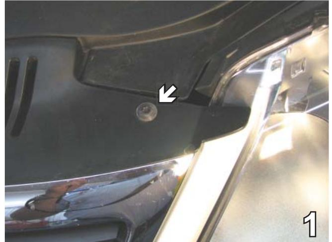
1. On the top edge of the fascia remove the screw in the corner with a T-25 Torx socket. Do this on both sides and set aside for later reinstallation.
