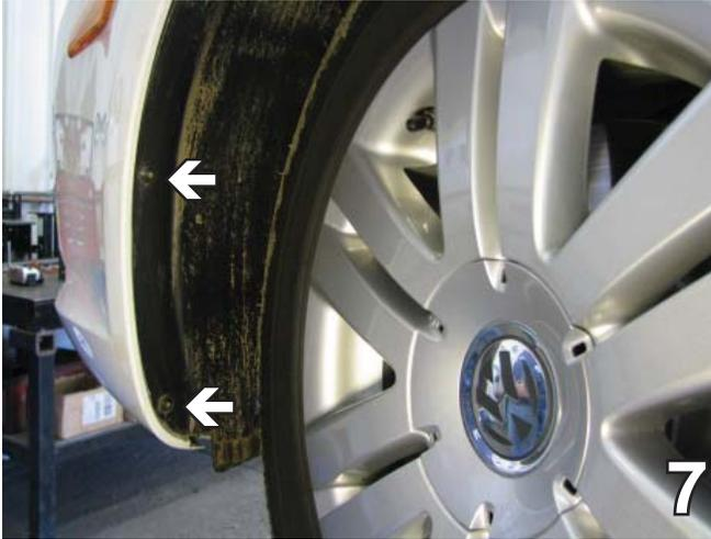
7. Just forward the front tire in the wheel well, remove two T-25 Torx screws. Set screws aside to reinstall later.
