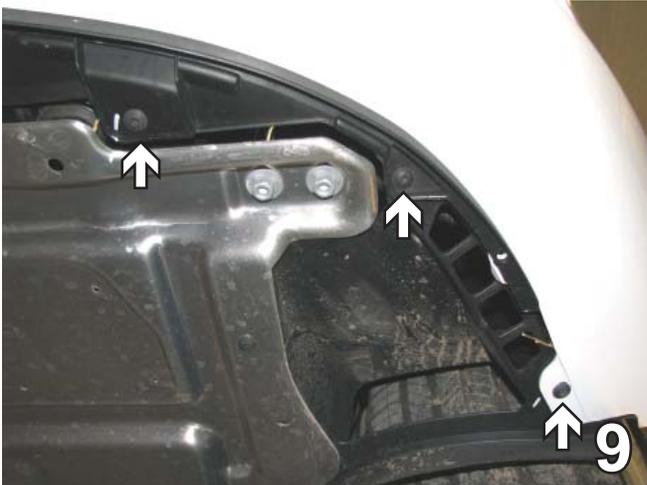
9. Under the fascia are nine Torx bolts that need to be removed with a T-25 Torx socket. Remove bolts and set aside for later installation.
