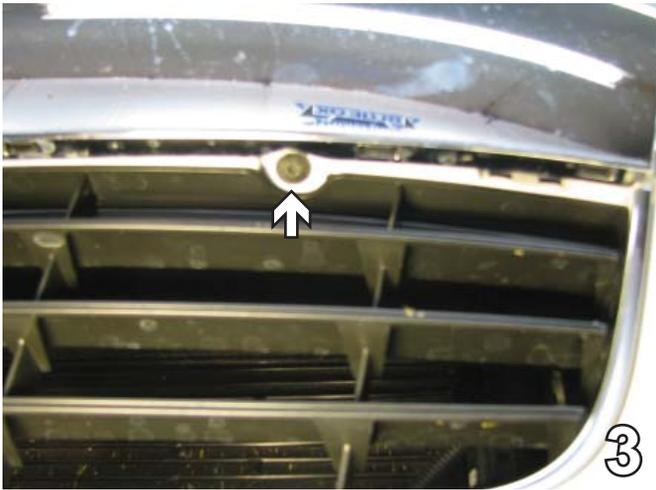
3. Using a T-25 Torx remove the two bolts holding the chrome. Set chrome and bolts aside for later reinstallation.
