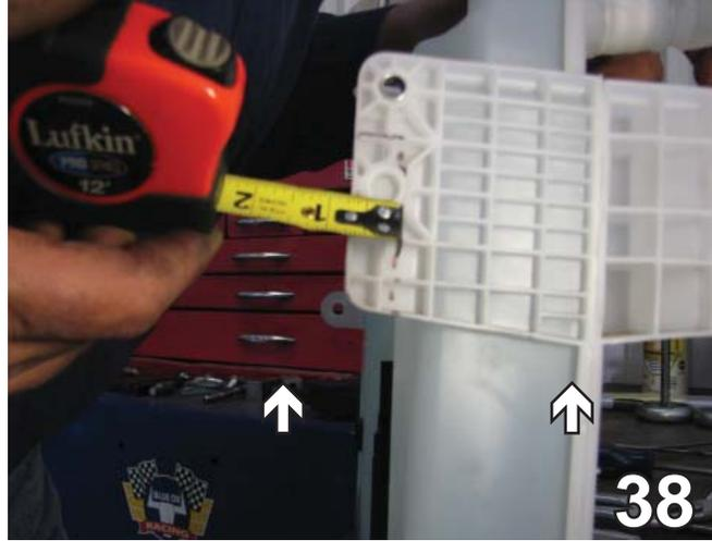
38. On the back side of the washer reservoir, mark a line 3/4" away from the back rib and 1 1/4" up from the bottom frame edge. Cut below the rib all the way down.
