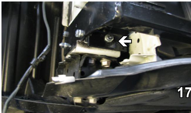
17. Insert a 3/8-16 x 1 1/2" hex bolt with 3/8" lock washer and 1/4" x 1" x 1" nut plate into the opening on the side of frame support. Tighten with Loctite Red. Do the same on the other side.
