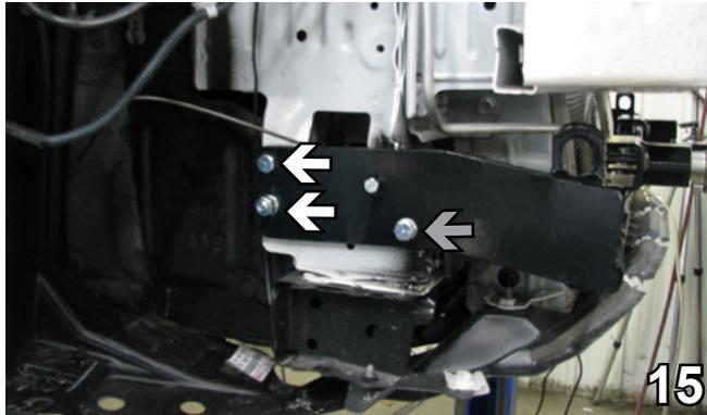
15. On the passenger side, the back two bolts (white arrows) are 3/8-16 x 1" hex bolts and 3/8" lock washers with 3/8-16 hex nuts. The front (grey arrow) is a 3/8-16 x 1 1/2" hex bolt with a 3/8" lock washer and 1/4" x 1" x 1" nut plate inserted through the opening above the baseplate. Tighten all bolts with Loctite Red.
