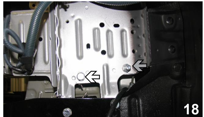
18. To give reinforcement to frame webbing, using the 13/32" drill bit, drill two holes, insert 3/8-16 x 1" hex bolts. In the front (white arrow) use 1/4" x 1" x 1" nut plates and in the back (grey arrow) use 3/8" lock washers with 3/8-16 hex nuts. Tighten with Loctite Red. Do this on both sides.
