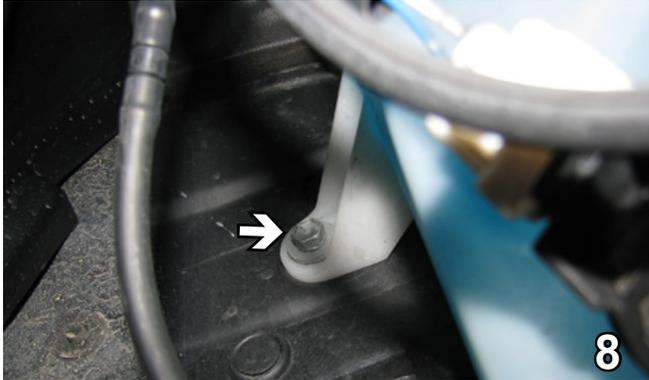
8. Using a 10MM socket, remove the bolt from between wheel well cover and left side of washer reservoir on the passenger side only. Disconnect all electrical and fluid lines, then remove reservoir and bolt. Set aside for later reinstallation.
