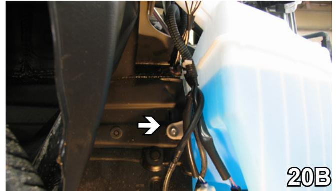
20. Attach top and left washer reservoir with #10-16 x 1" self drilling screws with 1/4" flat washers into frame. Reattach all wires and hoses.
