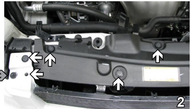
2. On the passenger side, using a flat screwdriver, remove five plastic push pins and with a 10MM socket, remove one metric bolt on the outside edge (grey arrow). Set push pins and bolt aside to be reinstalled later.
