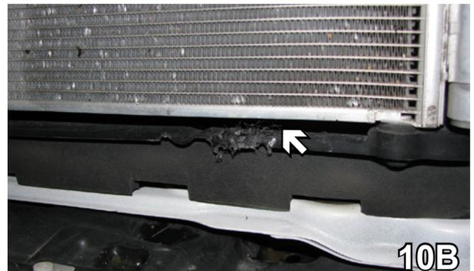
10. On the driver's side, remove the sensor and clip. Using a reciprocating saw, cut off the bracket flush with lower radiator support. Be sure not to damage radiator.
