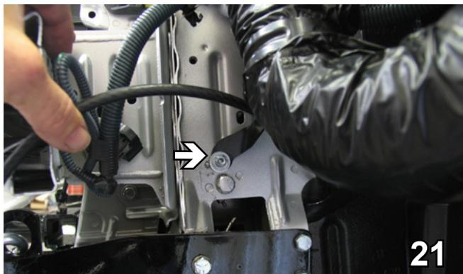
21. Reattach the vent tube using a #10-16 x 1" self drilling screw with a 1/4" flat washer.
