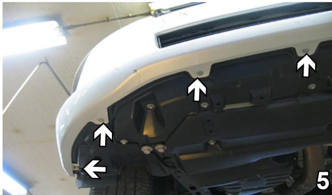
5. Remove eight metric bolts from lower edge of fascia all the way around using a 10MM socket. Pull fascia corners out to the side of the vehicle on both sides, then forward. Set aside fascia and bolts aside carefully for later reinstallation.
