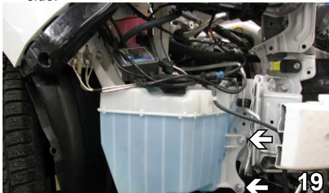
19. Reattach washer reservoir, use 6MM-1.0 x 30MM hex bolts and a 1/4" flat washer. In the top, use a 5/8" tube spacer and a 1/4" flat washer.
