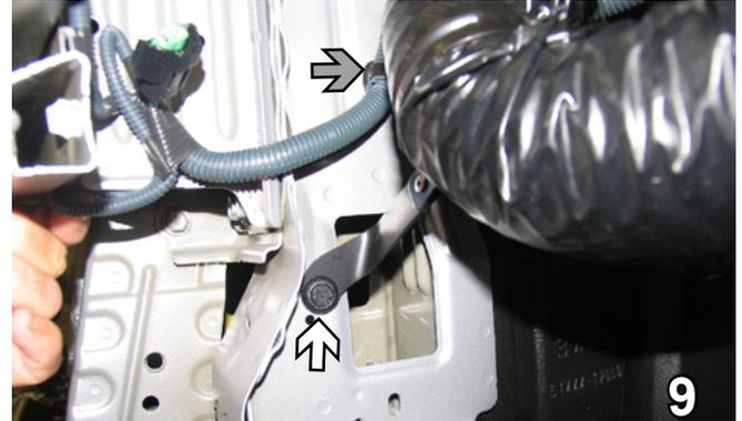
9. On the driver's side, using a flat screwdriver remove the push pin holding the vent tube. Also pull out the clip (grey arrow) from wire loom. Move the vent tube out of the way. Save the pin to reinstall later.
