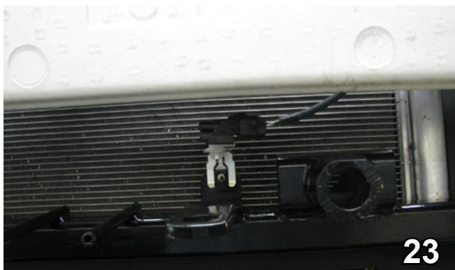
23. Put the temperature sensor back on the little plate in front of the radiator.
