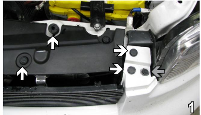
1. Using a flat screwdriver, remove four plastic push pins from the radiator cover driver's side and with a 10MM socket, remove one bolt from the outside edge (grey arrow). Set push pins and bolt aside to be reinstalled later.
