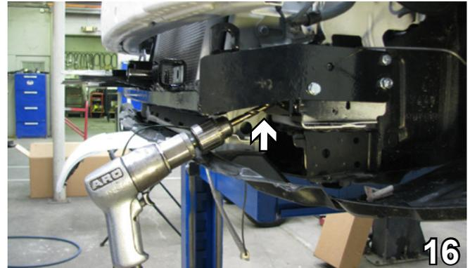
16. Using the 13/32" drill bit, drill at an angle one hole using the baseplate as a template into the front of lower frame support. Do this on both sides.
