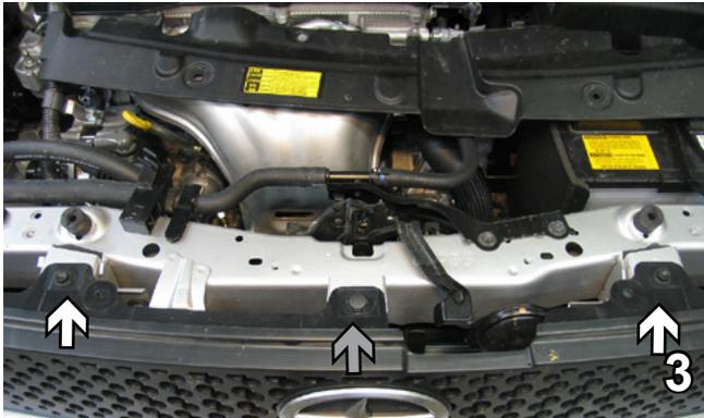
3. Above the grill, remove the cover. Using a 10MM socket, remove two metric bolts. Using a flat screwdriver, remove push pin from the center (grey arrow). Set cover, bolts and pin aside to be reinstalled later.
