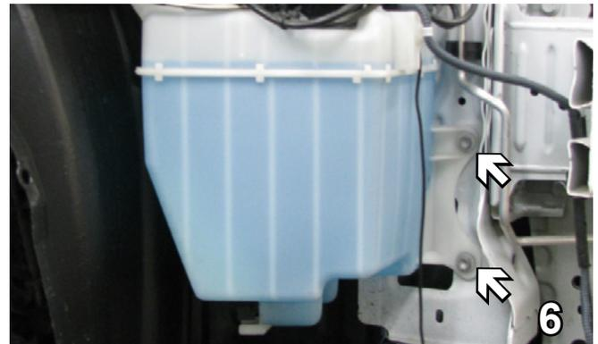
6. Using a 10MM socket, remove two bolts from the right side of the washer reservoir on the passenger side only. Set bolts aside for later reinstallation.
