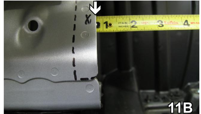
11. Using a reciprocating saw, cut a notch 3 1/2" long by 3/4" in lower frame support webbing. Do this on both sides. (Vertical cut should be flush with the side of support.)
