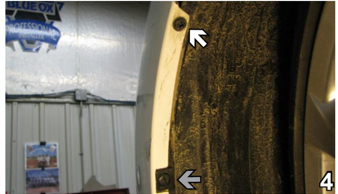
4. Using 10MM socket, remove one metric bolt just forward of the front tire on bottom side of fascia. Using a flat screwdriver, turn the screw pin (grey arrow) 90° and the screw will pop out. Do this to both sides of vehicle. Set bolts and pins aside to be reinstalled later.
