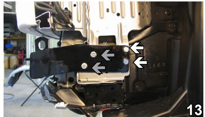
12. On the driver's side, slide the baseplate into the notch we cut out and as far back as possible, it should be flush with back webbing. Adjust to a level position with the vehicle and clamp with large vise grips. Do this on both sides. Using the baseplate as a template with a 13/32" drill bit, drill all four holes.
