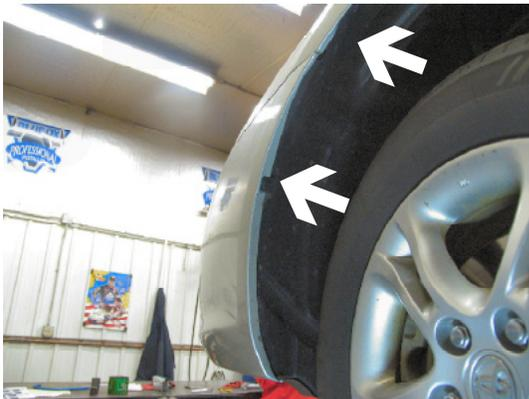
3. Just forward of front tires, on fascia and wheel well edge is one plastic screw to remove, on both sides and one push pin just above front tire on edge of wheel well, on both sides.
