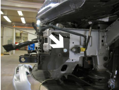
6. Hold base plate in place and align back holes with existing holes on frame, on both sides. Then insert 1/2-13 Whiz nut, with 10 inch wire, into opening on frame end to align with existing lower back hole of base plate, tighten 1/2-13 hex bolt and lock washer, on both sides. While maintaining a level position for the attachment tabs, tighten all bolts. **Be sure and use Loctite red on all bolts before tightening. Tighten all bolts according to torque chart in the General Instruction sheet.**
