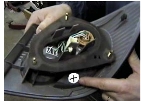
Location of the BX8869, on the bottom of the driver's side tail light assembly.
