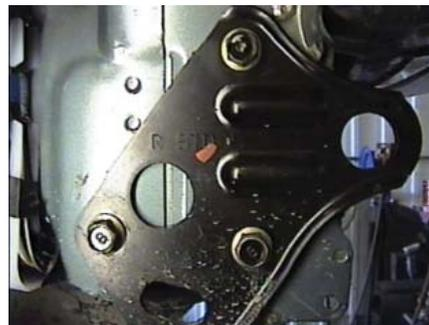
6. Remove passenger's side tie down bracket with the 14MM socket.
