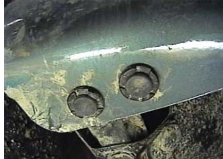
2. Just forward of front tire, on lower fascia corner, remove the two push pins, both sides.
