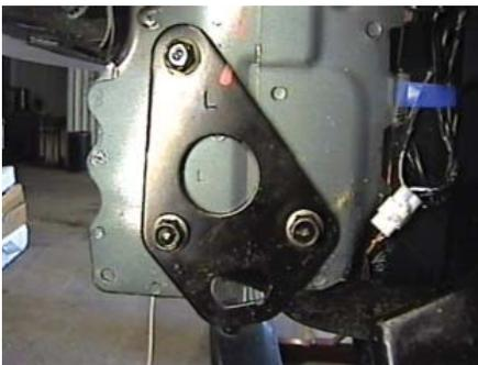
5. Using the 14MM socket, remove three metric bolts from driver's side tie down bracket. Tie down brackets will not be reinstalled. Metric bolts will be used later to install baseplate.
