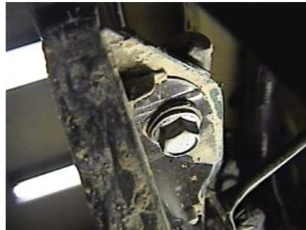
4. Using the 10MM socket, remove the metric bolt inside wheel well on upper fascia corner, both sides. Pull fascia forward and set aside.
