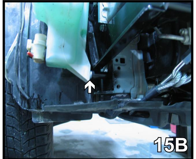
15. Reinstall the washer reservoir using 6MM -1.0 x 30MM hex bolts, 1/4" flat washers and 1 1/2" pipes in the two top holes. In the bottom hole, use a 6MM-1MM X 80MM hex bolt, 1/4" flat washer and 2 1/2" tube.
