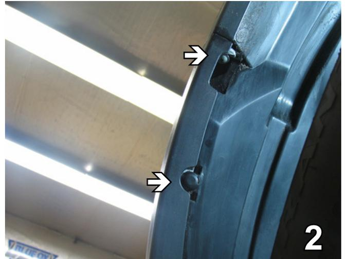
2. Just forward of the front tire, inside the wheel well, remove pushpin and Phillips screw. Do this to both sides of the vehicle. Set push pins and screws aside to reinstall later.
