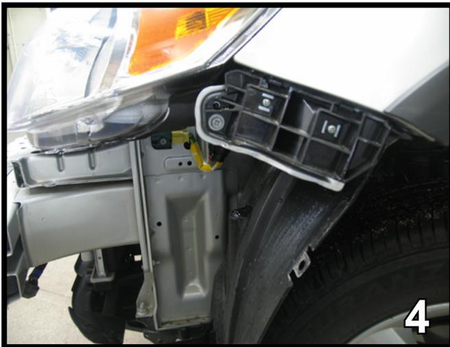
4. To remove fascia, pull it out to the side and forward a little bit. Once fascia is forward there are two clips on top to be removed by pushing in on the fascia and lifting up on the clips to get them over the stops. Set fascia aside carefully to reinstall later.
