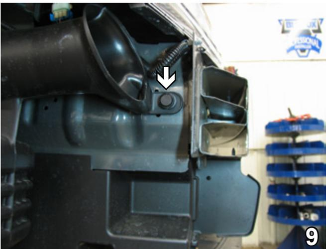
9. On the passenger's side, remove one (1) pushpin from the air baffle. Set pushpin aside to be reinstalled later.
