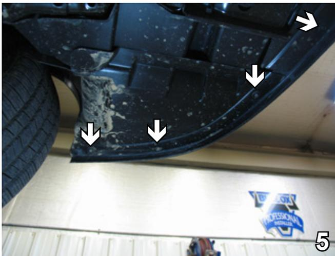
5. Using the 7MM socket, remove four (4) metric bolts from inside front edge of fascia. Do this to both sides of the vehicle. Pull fascia forward to remove. Set bolts and fascia aside to be reinstalled later.
