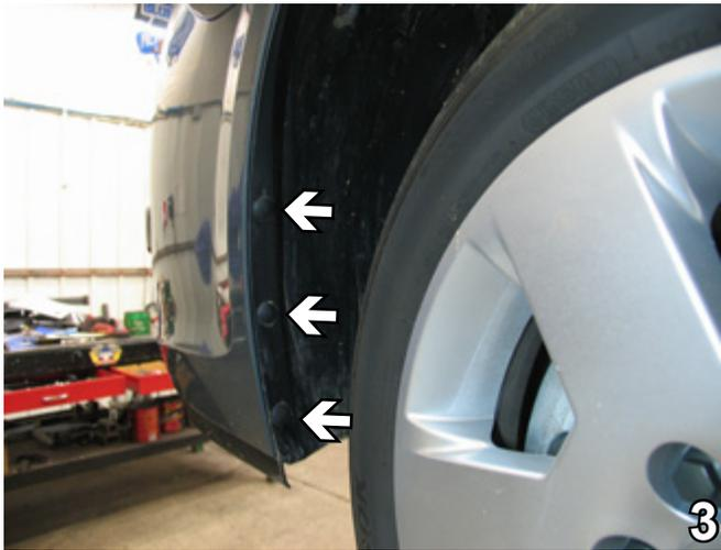
3. On outside edge of wheel well, remove three (3) christmas tree pushpins. Do this to both sides of the vehicle. Set pushpins aside to be reinstalled later.
