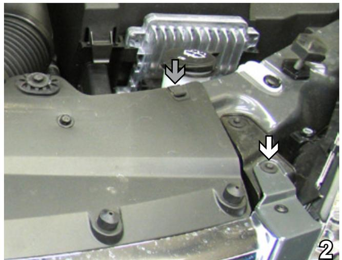
2. Using the 7MM socket, remove one (1) metric bolt from the top corner of fascia (see white arrow). On the top corner of radiator cover, remove one (1) clip (see grey arrow) using the flat screwdriver. Do this to both sides of the vehicle. Pull radiator cover forward to remove. Set bolts, clips and radiator cover aside to be reinstalled later.
