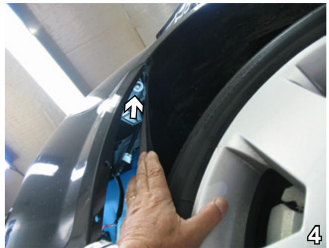
4. Push wheel well cover aside to remove one metric bolt using the 10MM socket. Do this to both sides of the vehicle. Set bolts aside to be reinstalled later.
