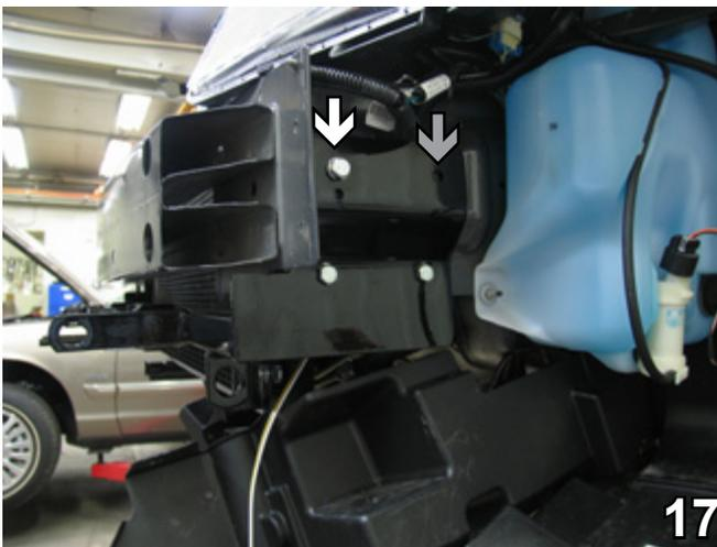
17. On the driver's side, insert 3/8" nut plate through opening in the bottom of the frame rail and align to the upper front hole (see white arrow). Install 3/8"-16 x 1-1/4" hex bolt with 3/8" lock washers and tighten to nut plate. Reinstall horn bracket to upper back hole using 6MM hex bolt, 1/4" lock washer and 1/4" flat washer (see grey arrow). Trim excess nut plate wire.
