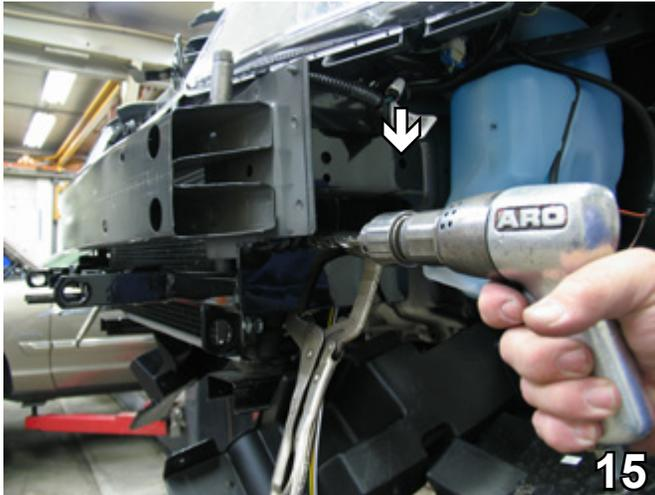
15. On the driver's side, align the upper back hole of the baseplate with the existing horn bracket hole and clamp in place with the vise grips. Using the baseplate as a template, drill the three (3) remaining holes into the frame using the 13/32" drill bit.
