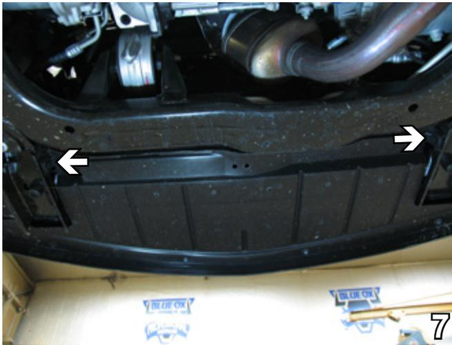
7. Remove two (2) pushpins from bottom of belly pan. Pull belly pan forward to remove. Set pushpins and belly pan aside to be reinstalled later.
