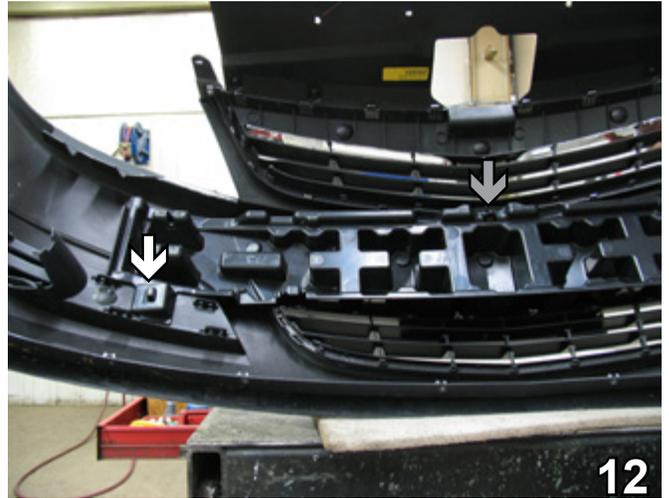
12. Lay fascia face down on a smooth, flat surface. Press in to release clip on the side of fascia support (see white arrow). Do this to both sides of fascia support. Press back to release clip on center of fascia support (see grey arrow). Pull fascia support to remove.
