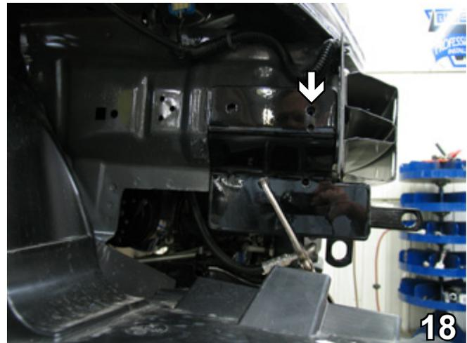
18. On the passenger's side, align the upper front baseplate hole with the existing air baffle hole and clamp in place with the vise grips. Using the baseplate as a template, drill four (4) holes into the frame using the 13/32" drill bit.
