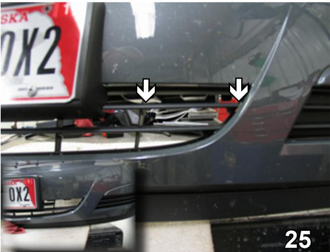
25. Align the fascia to its original position and, using the hack saw blade, trim necessary openings in the grille style for the attachment tabs. Do this to both sides of the vehicle.
