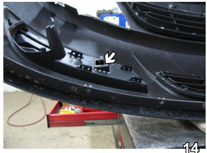
14. Using the utility knife, remove the tab from the back corner of the fascia. Do this to both sides of vehicle.
