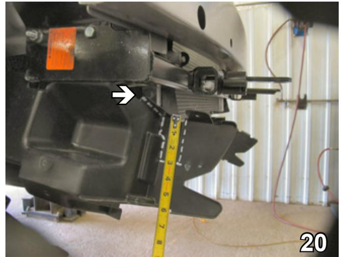
20. Mark the passenger's side of the air dam from the back portion of lip diagonally to the bend and down 3 inches around the contour of the air dam mold. Then mark straight down from the air dam tab three inches and horizontally back to the air dam contour and trim this area with the utility knife.
