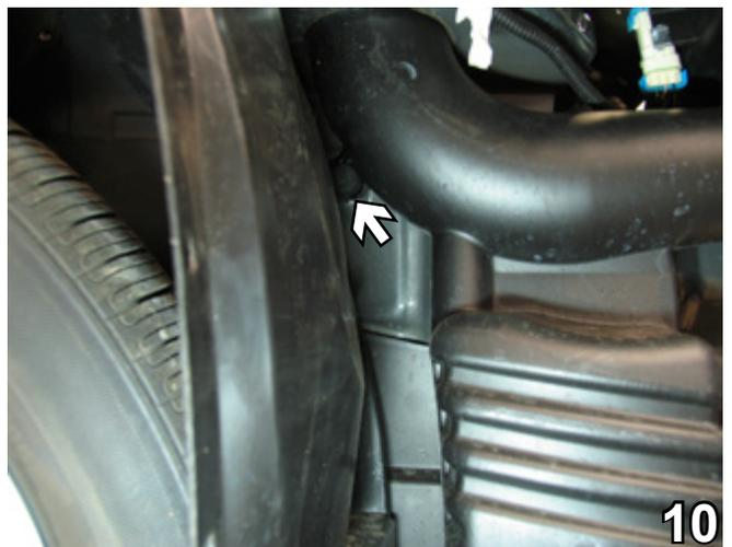
10. On the passenger's side, remove one (1) pushpin between the air baffle and the wheel well. Pull air baffle down to remove. Set pushpin and air baffle aside to be reinstalled later.
