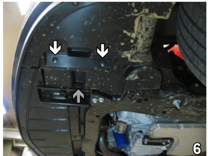
6. Remove two (2) christmas tree pushpins (see white arrows) and one (1) regular pushpin (see grey arrow) from the lower corner of belly pan. Do this to both sides of the vehicle. Set pushpins aside to be reinstalled later.
