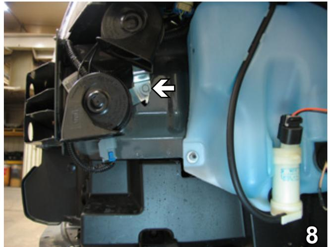
8. On the driver's side, disconnect electrical from the horn. Using the 10MM socket, remove one (1) metric bolt from the horn bracket. Set bolt and horn bracket aside to be reinstalled later.
