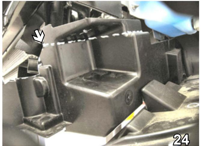
24. On the driver's side, approximately 1" from the top of the air dam, cut horizontally from the front of the air dam to the back.
