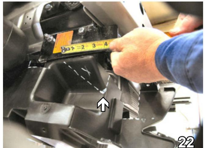
22. On the passenger's side of the air dam, just behind the tab, mark 3" down and 2" horizontally. Then mark upwards, following the contour of the air dam, to the top of the air dam and trim away this area with the utility knife.
