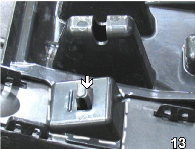
13. After removing fascia support, use the utility knife to remove the clip on both corners of fascia support.
