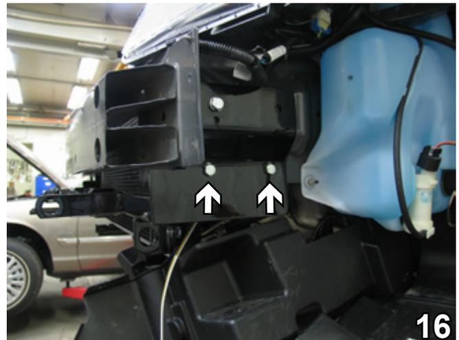
16. Install 3/8"-16 x 1-1/4" hex bolts with 3/8" lock washers and 3/8"-16 hex nuts to lower two (2) holes.
