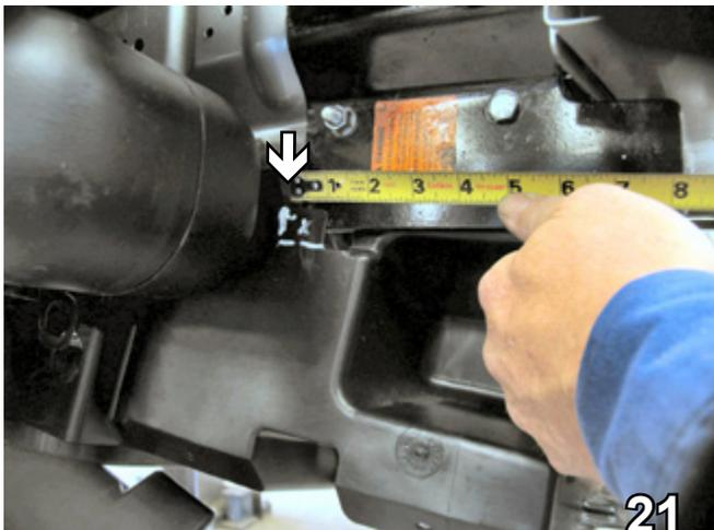
21. On the passenger's side upper rear of the air dam, use the utility knife to make a 1" horizontal cut level with the opening next to the air dam then trim vertically to remove this portion of the air dam.
