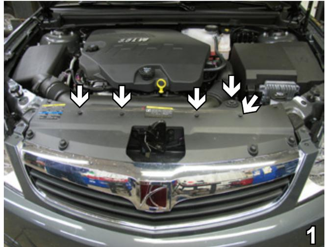
1. On top of the radiator cover, remove five (5) metric bolts using the 10MM socket. Set bolts aside to be reinstalled later.
