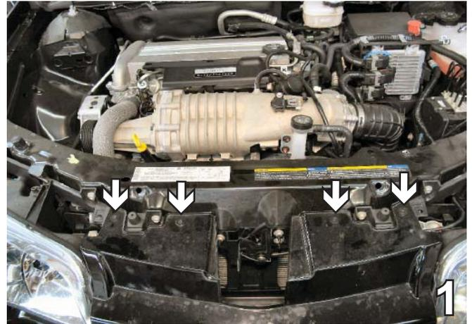
1. Using a 7MM socket, remove four metric bolts from the top side of the fascia. Set bolts aside to be reinstalled later.
