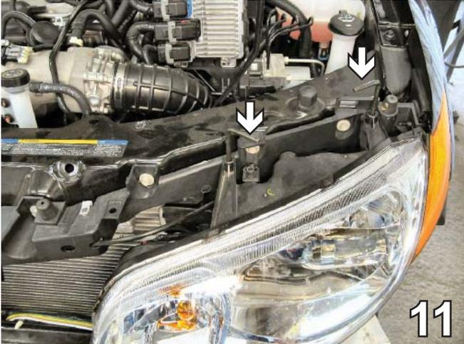
11. Rotate the headlight assembly rods until they point toward the front of the vehicle, pull up and out to remove them. Pull headlight assembly forward and disconnect electrical connections. Set rods and headlight assembly aside to be reinstalled later. Do this to both sides of the vehicle.
