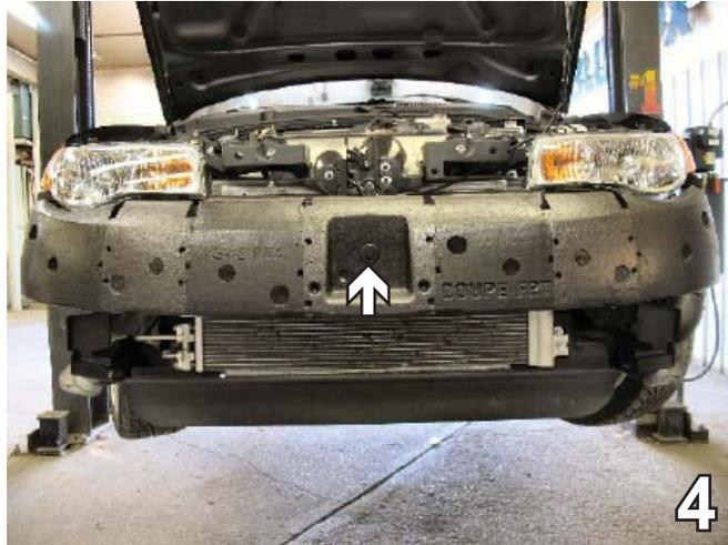
4. Remove one pushpin from the Styrofoam bumper. Set Styrofoam bumper and pushpin aside to be reinstalled later.
