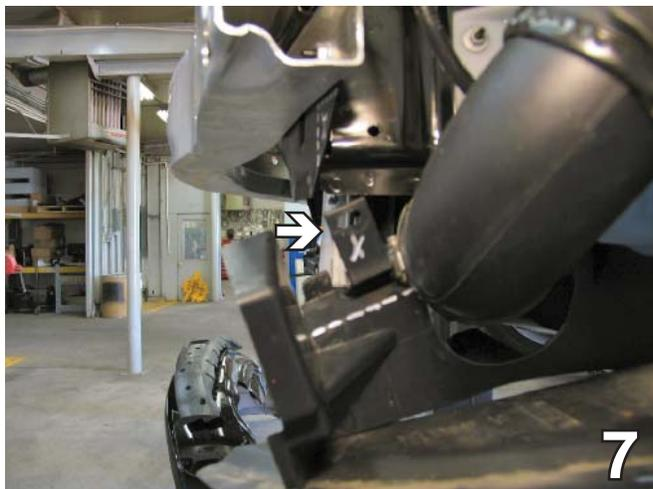
7. On the driver's side, remove one pushpin from between the metal bumper and the frame rail. Using a utility knife, cut along the bend to remove the tab of the air dam.
