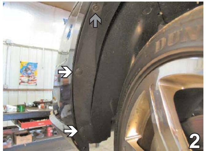
2. Inside the wheel well, just forward of the front tire, use a 7MM socket to remove one metric bolt, as indicated by the grey arrow in the photo above. Remove two pushpins, as indicated by the white arrows in the photo above. Set bolt and pushpins aside to be reinstalled later. Do this to both sides of the vehicle.
