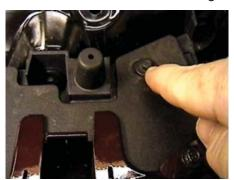
1. Remove the four metric bolts from the top side of fascia using the 7MM socket. Quad coupe model will not have black cover.
