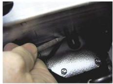
4. Using the bottom edge of the metal bumper as a guide, mark the front of the bumper bracket with a scribe toward the inside of frame end, both sides.
