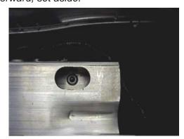
**5.** Remove six metric bolts from metal bumper using the 13MM socket, set metal bumper aside.
