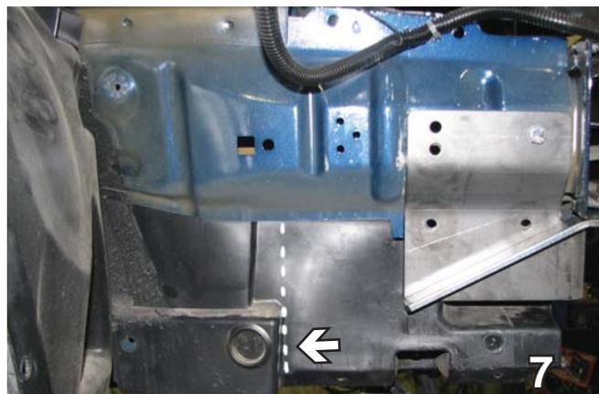
7. On the passenger side, using a utility knife, cut the plastic straight up next to the extended tab, as shown, and remove for nut plate insertion.
