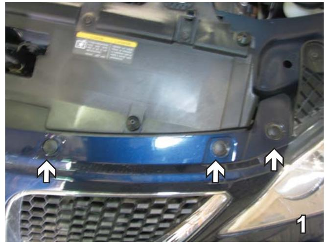
1. Remove the six push pins, three on each side, from the top edge of fascia just between headlight assemblies. Set pins aside to be reinstalled later.
