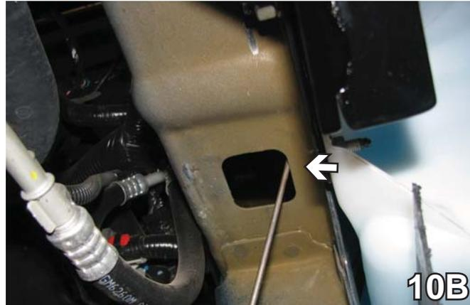
10. Using the baseplate as a template, drill a hole into the bottom of metal bumper with the 13/32" drill bit, both sides. Insert the 3/8" nut plate with the 12" wire into the open end of metal bumper to align with drilled hole, tighten 3/8-16 x 1 1/2" hex bolt and 3/8" lock washer with the 9/16" socket, both sides. Be sure and use loctite red on all bolts before tightening. Tighten all bolts according to torque chart in the General Instruction sheet.
