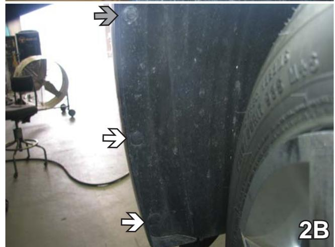
2. Remove three christmas tree push pins (white arrows) from the edge of wheel well, just forward of front tire. Using a 7MM socket, remove one metric bolt (gray arrow in 2B) half way up. At the top, using a 10MM socket remove another metric bolt (gray arrow in 2A). Do this on both sides. Set pins and bolts aside to reinstall later.
