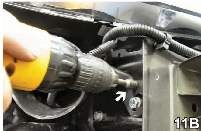
11. Remove rubber grommet from the front bolt location on the air baffle. Reinstall the air baffle on the passenger's side to its original position, using the existing metric bolt and lower push pin. Slide front bolt location over the top of front bolt of baseplate. Using the 5/16" nut driver and drill, install the #10 x 1 self drilling screw through air baffle webbing and into frame. This will help to stabilize the air baffle. Do not drill into baseplate.
