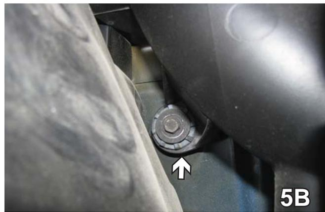
5. On the passenger side, remove the push pin from the front of the air baffle. Using a 10MM socket, remove one metric bolt from the back. Set assembly aside to be reinstalled later.
