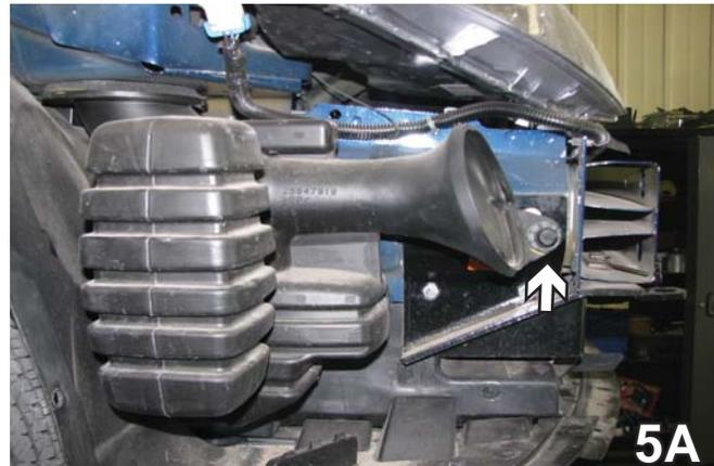
4. Using the 10MM socket, remove metric bolt from horn bracket on the driver's side and set assembly aside to be reinstalled later.
