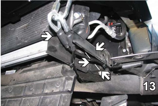
13. Attach permanent baseplate safety cables to the convenience link on the baseplate. Wrap the cables around the vehicle frame. Additional options may interfere with suggested mounting, in this case secure the cables to a solid piece of the frame as described in instructions included with the permanent baseplate safety cables. Be sure the safety cables do not rub against any hoses or moving parts. Do this to both sides of the vehicle.
