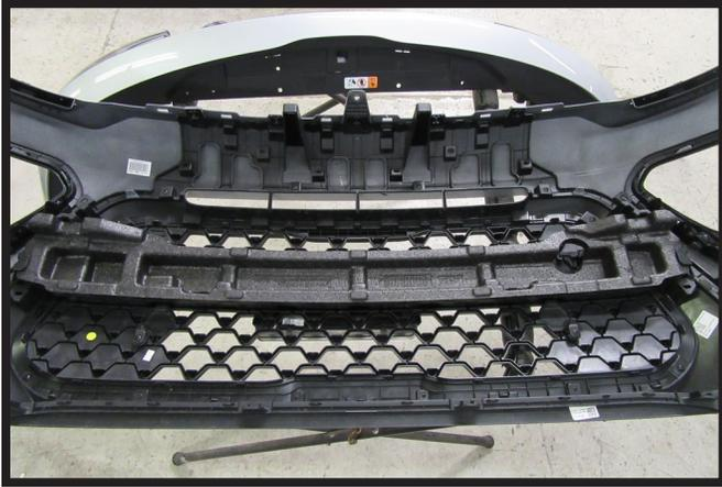
7. Remove the Styrofoam from the back of the fascia by releasing the tabs holding it in place on each side. This will not be reinstalled.
