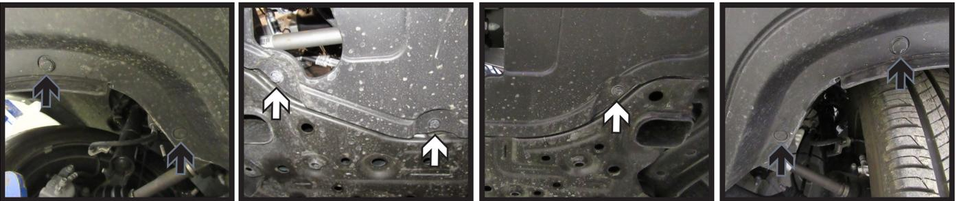
6. Using a 10MM socket, remove the seven (7) bolts (white) from the belly pan. There are four (4) in the front and three (3) in the back. Using a 14MM socket, remove the one (1) plastic bolt (gray) from the belly pan. Then remove the four (4) push pins (black), two (2) from each side. Remove belly pan and set aside to be reinstalled later.
