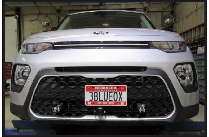
16. Hold the fascia as close to its original position, mark and trim the fascia around the convenience links and attachment tabs. Reinstall the belly pan and fascia.
