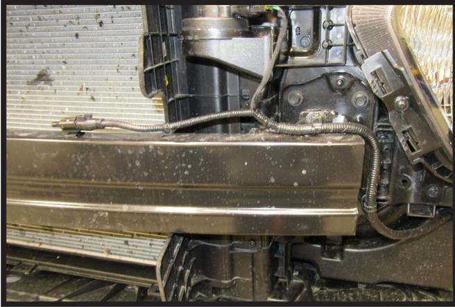
4. Unclip the temperature sensor wire loom from the bumper on the driver side of the vehicle. Set aside to be reinstalled later.
