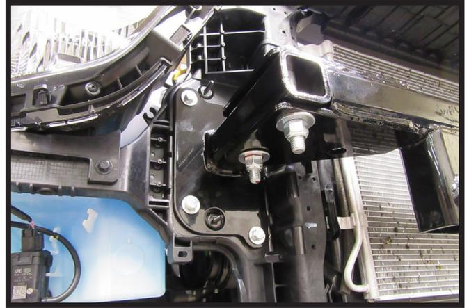
12. Tighten the two (2) 1/2" frame bolts and the eight (8) 8MM bolts on the front of the baseplate. Install the remaining hardware to the four (4) 1/2" cross member bolts and fully tighten.
