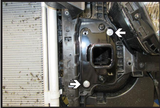
9. Start the two (2) 8MM bolts with hardware as shown. Do this on both sides of the vehicle.
