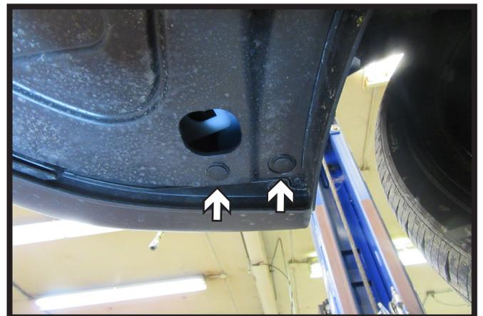
Remove fascia by lifting and pulling starting on the side to release clips along each side as well as the center. Set fascia aside to be reinstalled later.
