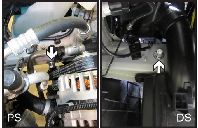
10. Start the two (2) 1/2" bolts with hardware, one (1) on each side, on the inside of the frame as shown. On the driver side this can be accessed from the underside of the vehicle and from above on the passenger side. When tightening the bolt on the passenger side, it is easier to do this from the underside of the vehicle.
