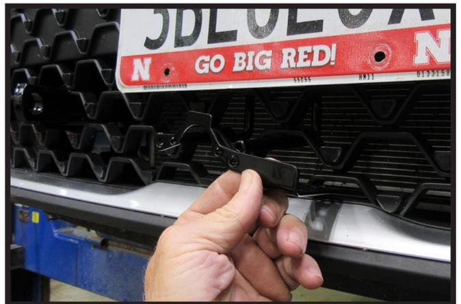
14. **Optional Breakaway:** Attach breakaway bracket to the electrical rods and trim fascia as needed.
