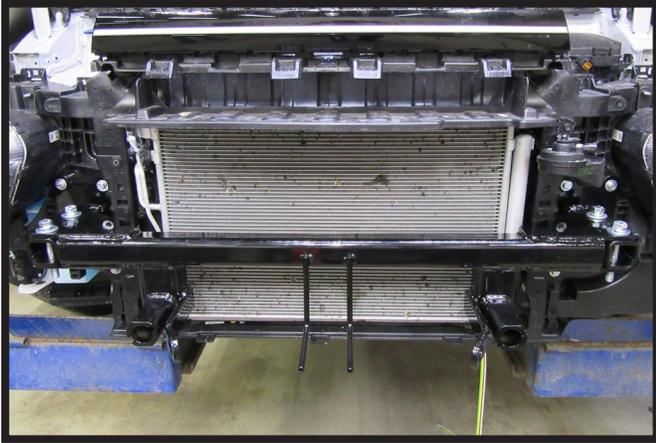
11. Start the remaining four (4) bolts, two (2) on each side to the front of the baseplate. Set the cross tube onto the side brackets. Place the four (4) 1/2" bolts with flat washer and lock washer into holes. Do not add hardware to the bottom of bolts.
