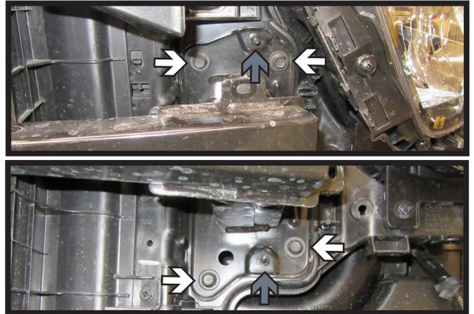
5. Using a 13MM socket, remove the four (4) bolts (white) from the bumper. Then using a 10MM socket, remove the two (2) bolts (gray) from the bumper. Do this on both sides of the vehicle. Remove bumper and set aside, it will not be reinstalled later.
