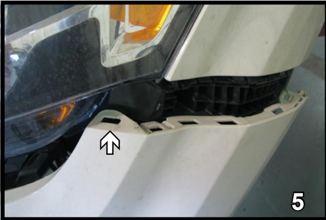
5. The fascia is then ready to be removed from the vehicle by grabbing in front of the tire, lift and pull the fascia ends out to the side to release and then pulling it forward. Use a screwdriver to pop the fascia over the knob at the end (white arrow). Do this to both sides of the vehicle. Set fascia aside carefully.
