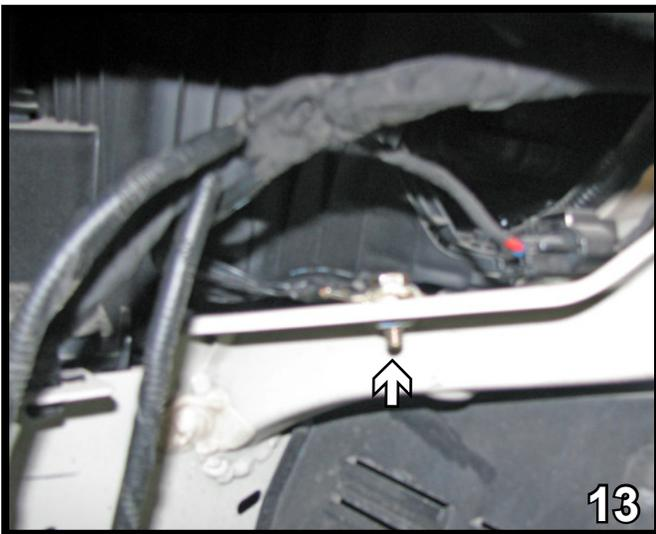
13. On the driver's side, the two ground wires need to be moved. Drill a 1/4" hole above. Attach both wires to the hole with 1/4-20 x 1" hex bolt and 1/4-20 whiz hex nut.
