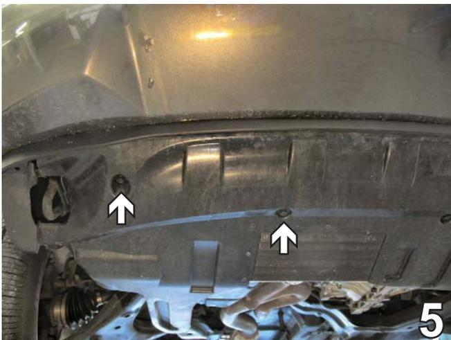
5. Using a 12MM socket, remove four metric bolts from the belly pan. Do this to both sides of the vehicle, the passenger's side is shown. Set belly pan and bolts aside to be reinstalled later.
