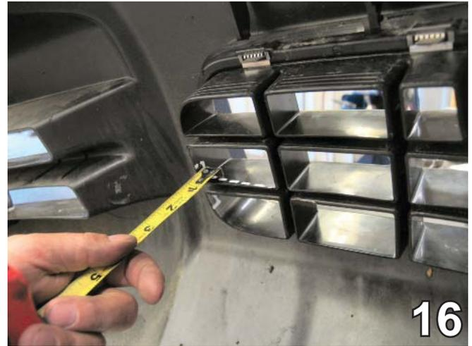
16. On the back side of the fascia, locate the openings closest to the grille edge. On the middle opening, cut in 1/2" and down, angling the cut so that it continues to the opposite edge of the opening. On the lower far left opening, cut in 1/2" and then upward, angling to the opposite edge also. Do this to both sides of the vehicle.
