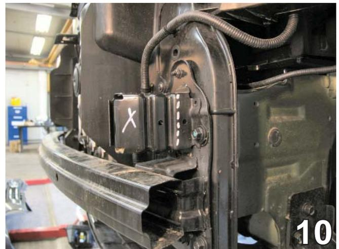
10. Using the reciprocating saw, trim away frame horn end by cutting vertically just forward of the bracket's rear bolt hole and horizontally along the entire width of the frame horn end and repeating to complete the rectangle. Do this on both sides of the vehicle, the driver's side is shown.
