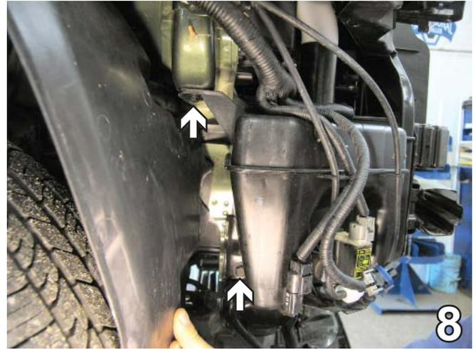
8. Press the wheel well cover toward the tire to expose two metric bolts to be removed using the 10MM socket. Unplug electrical connections, disconnect and plug water lines. Set bolts aside to be reinstalled later.
