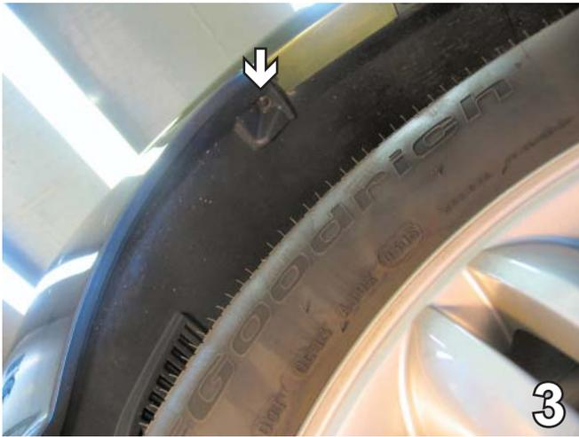
3. Just inside the wheel well, on the edge of the fascia, remove one metric bolt with an 8MM socket. Do this to both sides of the vehicle. Set bolts aside to be reinstalled later.
