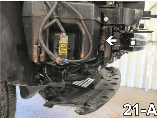
21. Remove one push pin between windshield washer reservoir and metal bumper (see 21-A). Insert four flat washers for additional clearance (see 21-B) and reinstall windshield washer reservoir to its original position.
