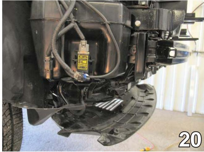
20. Reconnect electrical and water lines to windshield washer reservoir.
