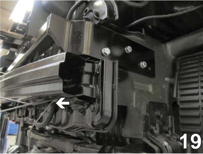
19. Insert three 3/8-16 nut plates through the lower bumper opening and align with drilled holes in the baseplate end plates. Insert the three 3/8-16 x 1 1/2" hex bolts and 3/8" lock washers and fasten to the nut plates. Do this to both sides of the vehicle, the driver's side is shown.
