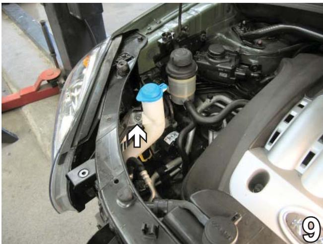
9. Using a 10MM socket, remove one metric bolt from the top spout of the windshield washer reservoir. Guide the windshield washer down and remove from the vehicle set aside to reinstall later. Set bolts and washer reservoir aside to be reinstalled later.
