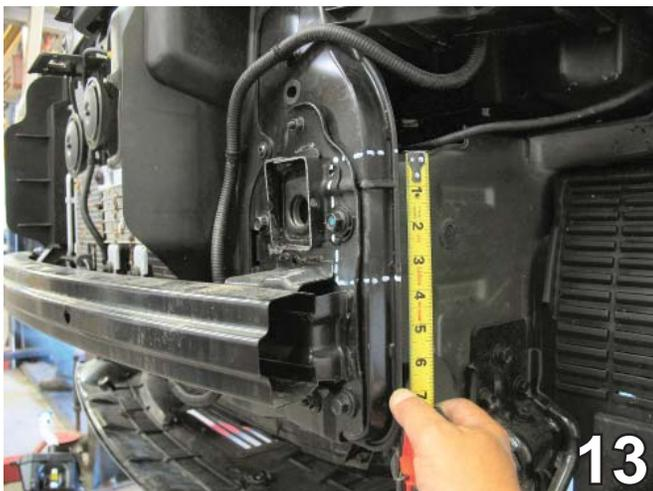
13. On the driver's side radiator support, mark and trim a section 3 1/2" high and flush with the frame rail to open the area for baseplate installation.
