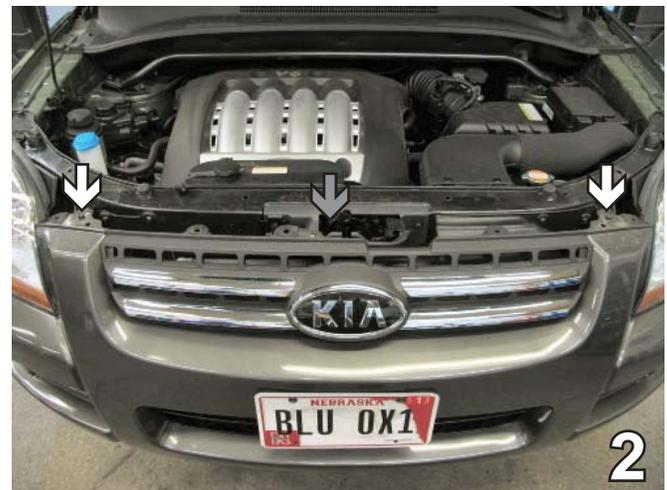
2. Using the 10MM socket remove two metric bolts from top corners of the fascia, see the white arrows in the photo above. Remove one Phillips screw from the top of the fascia, see grey arrow in the photo above. Set all aside to be reinstalled later.
