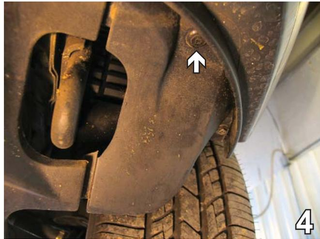
4. Just forward of the front tire, remove one Phillips push pin. Do this to both sides of the vehicle. Set aside to be reinstalled later.
