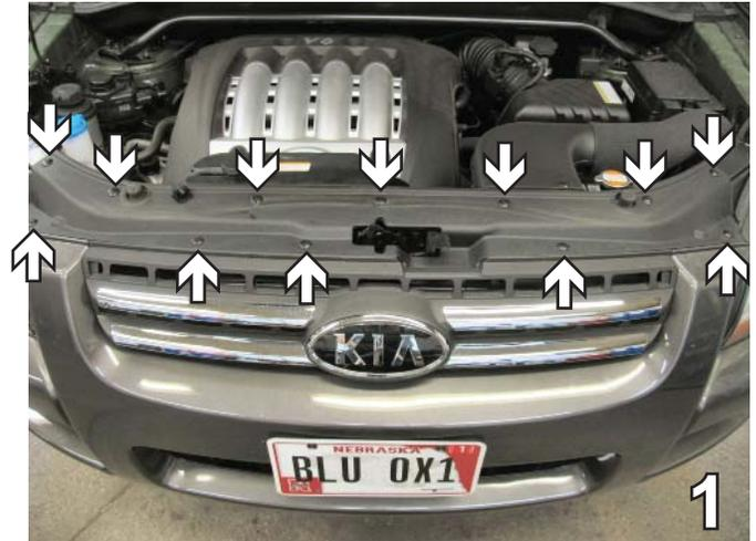
1. Remove 12 Phillips push pins from the top of the fascia. Then, remove the black plastic from the top of the fascia. Set push pins aside to be reinstalled later.
