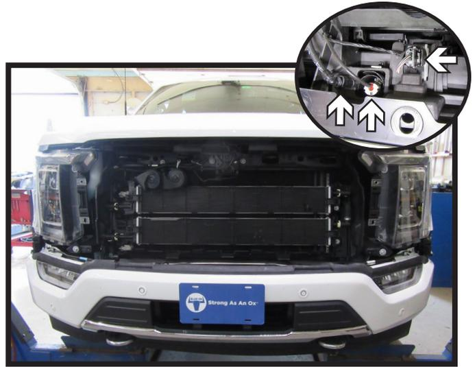
6. Lift the fascia cover and unplug the electrical connections (inset). Remove fascia and set aside to be reinstalled later.
