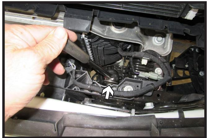
8. Coming from above the bumper, use a 21MM socket to remove the one (1) inside nut from behind the bumper. Do this on both sides of the vehicle.
