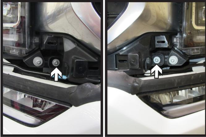
5. Using an 8MM socket, remove the two (2) inside bolts, one (1) on each side of the vehicle.
