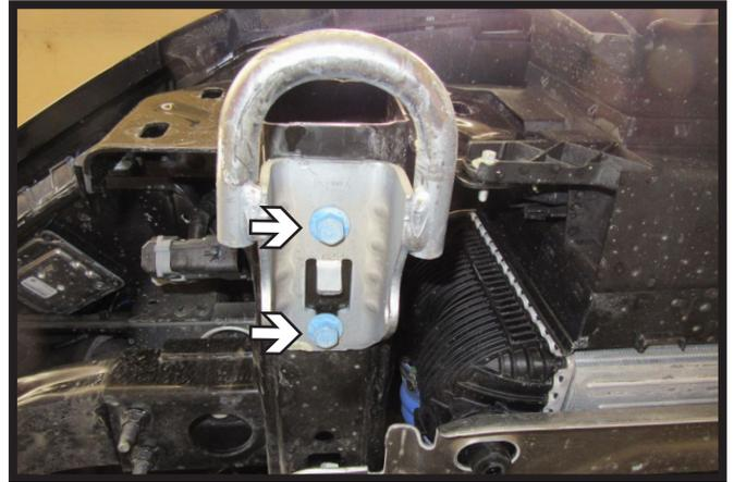
2. Using a 15MM socket, remove the two (2) bottom bolts from the tow hook. Remove tow hook and set aside, it will not be reinstalled. Do this on both sides of the vehicle.
