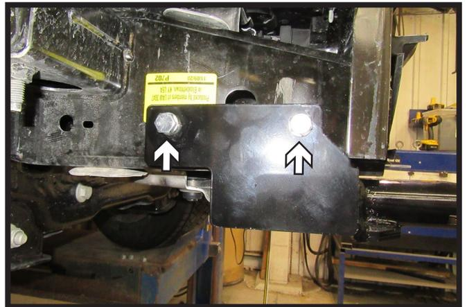
4. Using the baseplate as a template, use a 1/2" drill bit to drill two (2) holes through the frame of the vehicle. Install two (2) 1/2" bolts with hardware. Do this on both sides of the vehicle.
