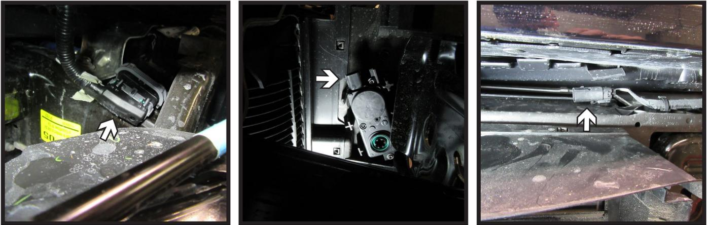
5. Start to remove the bumper. As the bumper is removed unplug the main electrical (left) and shutters (center) from passenger side of the vehicle. Then unplug electrical on top of the shutter housing (right) on the driver side of the vehicle. Set bumper aside to be reinstalled later.
