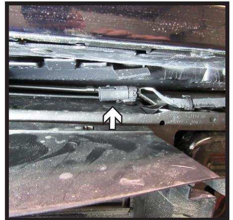
2. Start to remove the bumper. As the bumper is removed unplug the main electrical (left) and shutters (center) from passenger side of the vehicle. Then unplug electrical on top of the shutter housing (right) on the driver side of the vehicle. Set bumper aside to be reinstalled later.
