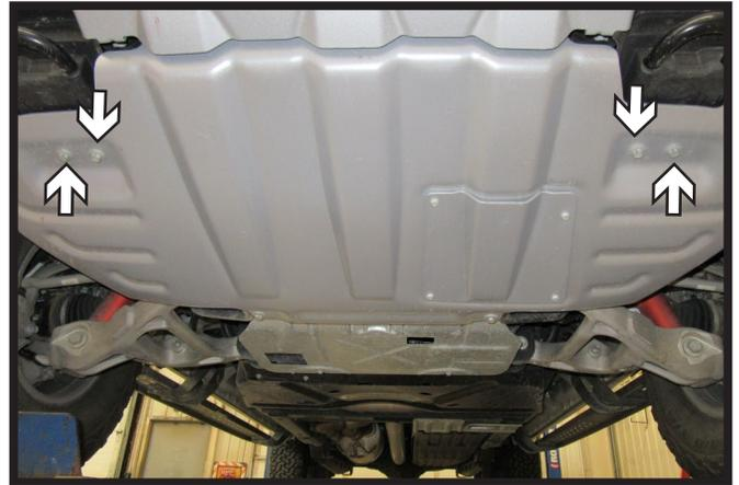
2. Using a 13MM socket, remove the four (4) bolts, two (2) from each side, under the tow hooks. Remove belly pan and set aside to be reinstalled later.
