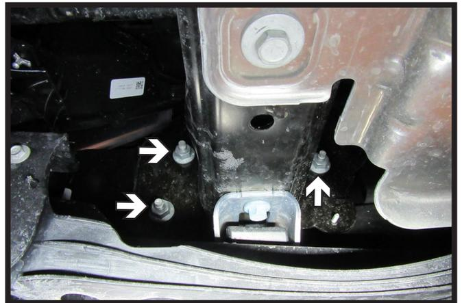
4. Using a 21MM socket, remove the three (3) nuts from behind the bumper. Do this on both sides of the vehicle.
