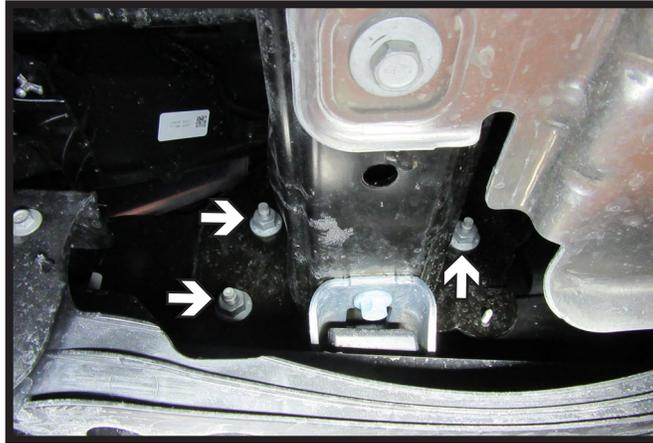
1. Using a 21MM socket, remove the three (3) nuts from behind the bumper. Do this on both sides of the vehicle.
