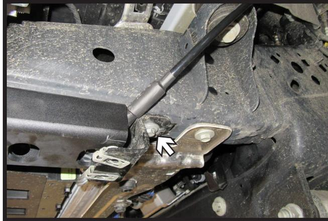
5. **Raptor Models:** Reinstall belly pan bracket before installing baseplate safety cables. Do this on both sides of the vehicle.
