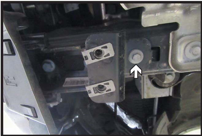
3. Using a 13MM socket, remove the one (1) bolt from the belly pan bracket. Remove bracket and set aside to be reinstalled later. Do this on both sides of the vehicle.
