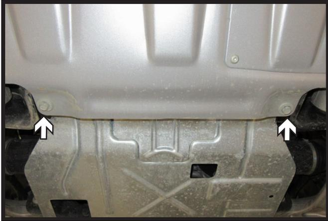
1. Using a 15MM socket, remove the two (2) bolts for the back of the belly pan.
