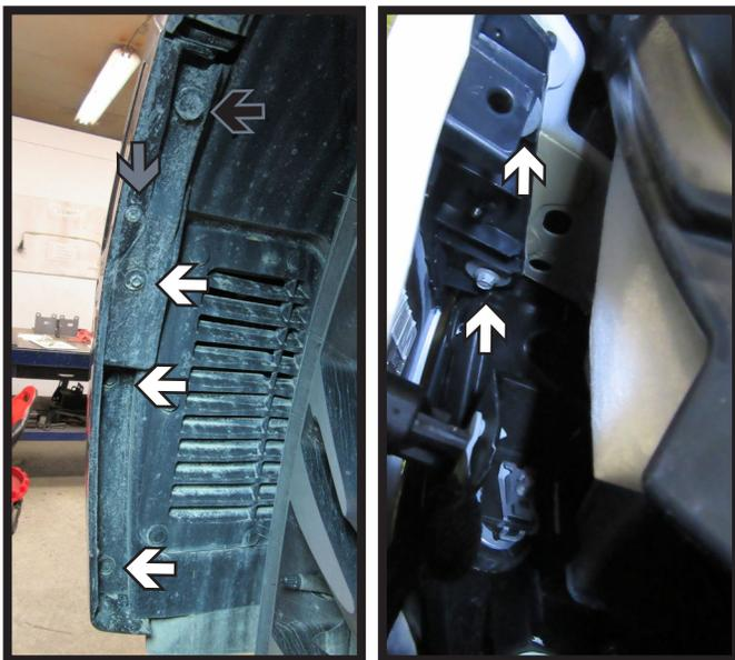
3. Using a 7MM socket, remove the three (3) bolts in front of the tire on the wheel well (white, left). Using a Phillips screwdriver, remove the one (1) screw (gray). Remove the one (1) push pin (black). Pull the wheel well cover back. Using an 8MM socket, remove the two (2) bolts (white, right). Do this for both sides of the vehicle.
