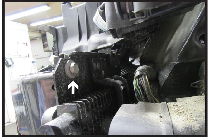
9. Using a 10MM socket remove the bolt holding the air bathel on the driver side of the vehicle and remove to be reinstalled later.
