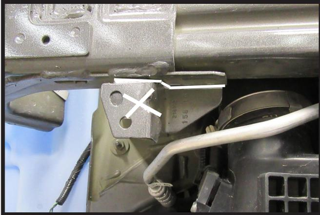
10. Using a reciprocating saw remove the indicated area on both sides of the vehicle so that it is flush with the bumper.
