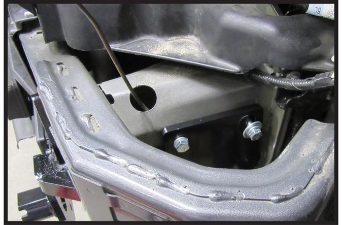
17. Line up the side plate and start the top two (2) 3/8" bolts but leave loose at this time. Use a 3/8" bolt with lock washer for the front hole. Use a 3/8" bolt with a flat washer and lock washer for the back bolt. Do this on both sides of the vehicle
