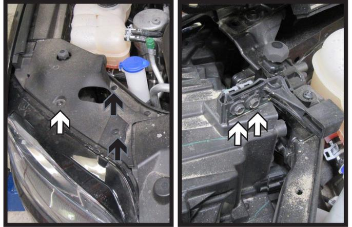
6. Using a T25 Torx, remove the one (1) screw from the plastic headlight cover (white, left). Remove the two (2) push pins (black). Pull the plastic cover up. Using a 10MM socket, remove the two (2) exposed bolts (white, right). Do this for both sides of the vehicle.
