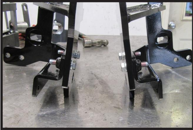
16. Before installing on the vehicle attach the Z bracket to the side plates using four (4) 3/8" bolts with lock washer.
