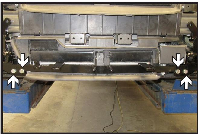
18. Using four (4) 1/2" bolts with lock washer and nylon lock nut attach the center cross bar to the side plates. Make sure that everything is level and tighten all bolts.
