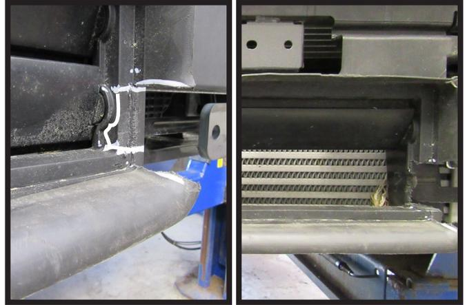
13. Then trim indicated area from on the shutter housing and remove the bottom shutter. Do this on both sides of the vehicle.
