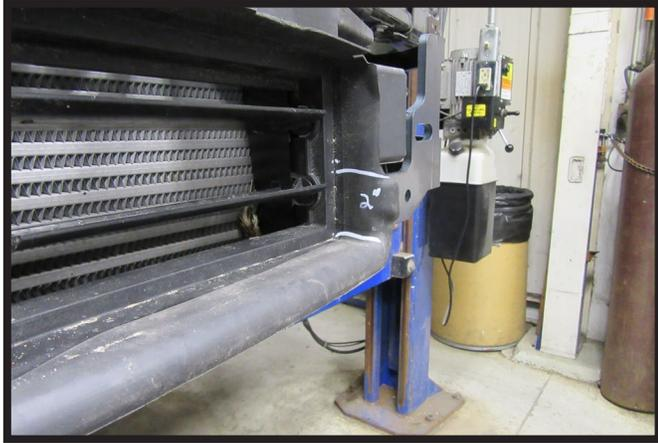
12. Measure 2" up from the bottom of the shutter housing and trim the indicated area. Do this on both sides of the vehicle.
