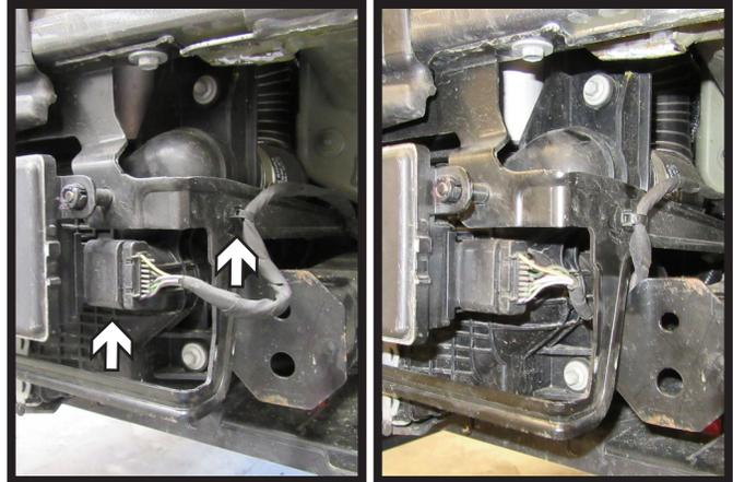
11. On the driver side of the vehicle unplug the electrical cable for the ACC sensor and remove the pin holding the electrical cable to the frame. Reroute the cable behind frame bracket and reattach pin and plug back into the ACC sensor.
