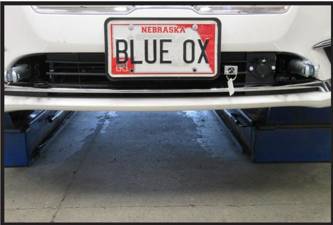
21. Hold the fascia as close to its original position, mark and trim the fascia around the convenience links and attachment tabs. Reinstall the headlights, fascia, and fascia cover.
