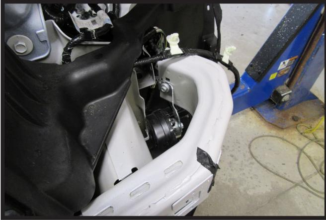
8. Using a 10MM socket, remove the one (1) bolt from the bumper horn and remove the bracket. Do this for both sides of the vehicle.
