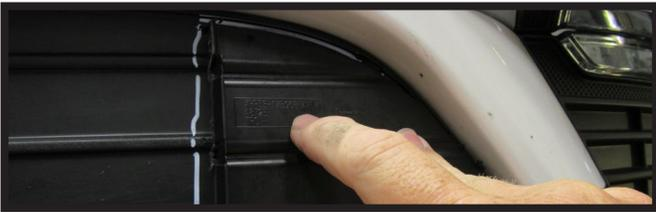
19. Using a reciprocating saw, trim the marked area on the passenger front of the fascia. Use this trimmed piece to mark and cut a similar shape on the driver side.
