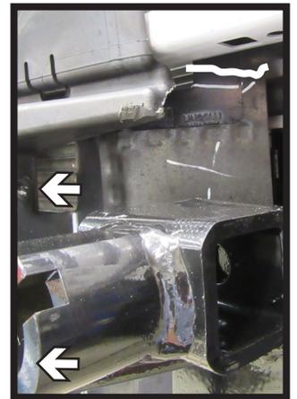
15. Using a reciprocating saw, trim the marked areas on both sides, behind the shutters. Remove two (2) push pins from both sides. (Bottom driver side pin not pictured)
