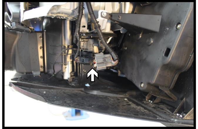
6. On the driver's side, locate the running lights main electrical cord. Disconnect the plug, and carefully remove the fascia.
