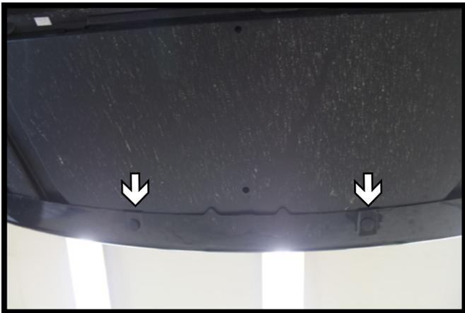
3. On the underside of the fascia, using a flat screwdriver, remove the two (2) pushpins from the front outer edge.
