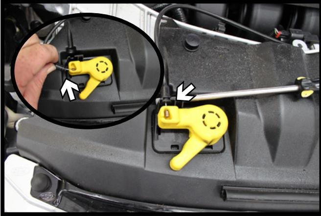
5. Using a flat screwdriver, pry the black hood latch cable out of the black mounting bracket (white arrow). Then rotate the wire left to release it.
