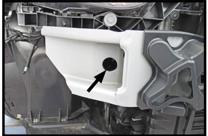
10. On the front bumper, using a 1-1/4" hole saw, slowly drill a hole centered vertically and horizontally on the flat area as shown. Do this on both sides of the vehicle. NOTE: The hole cut is used to place nut plates for future steps.
