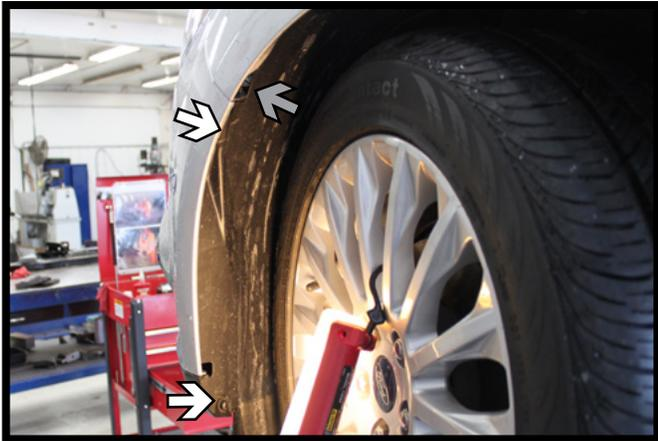
1. Using a T27 Torx, remove the two (2) screws from the driver's side front wheel well (white arrows). Using a flat screwdriver, remove the push pin from the driver's side front wheel well (gray arrow). Repeat this on the passenger's side.
