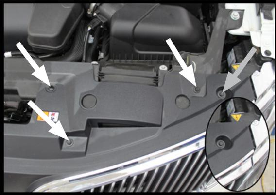
1. Using a 10MM socket, remove the six (6) bolts that are located in the front area, three (3) per side. There is one (1) push pin located on each side that will need to be removed also. NOTE: The bolt on the outer edge is not installed on 2012 models.
