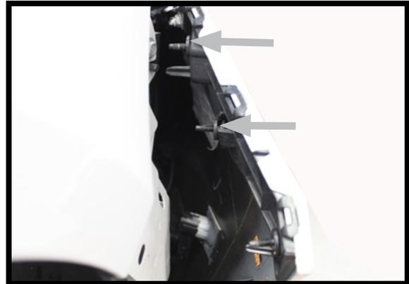
4. Unclip the fascia on both sides of the vehicle. Using a 10MM socket, reach inside, on the backside of the fascia remove three (3) bolts.
