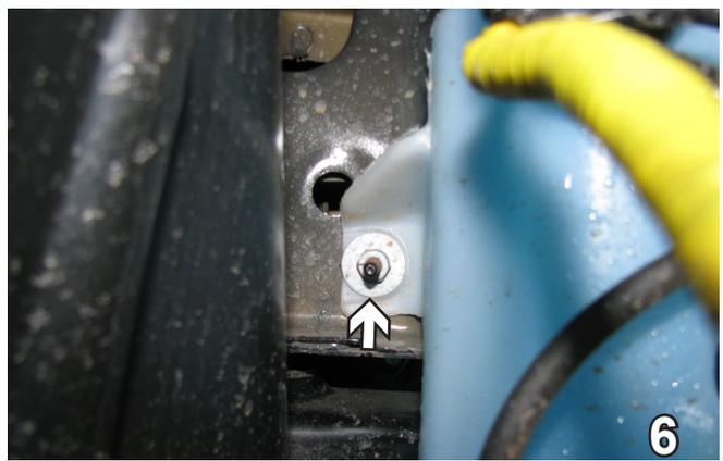
6. On the passenger side in order to remove the washer reservoir, remove the two (2) bolts from the left side using an 11MM socket. (Second bolt located on Step 7 gray arrow.) Set bolts aside to be reinstalled later.
