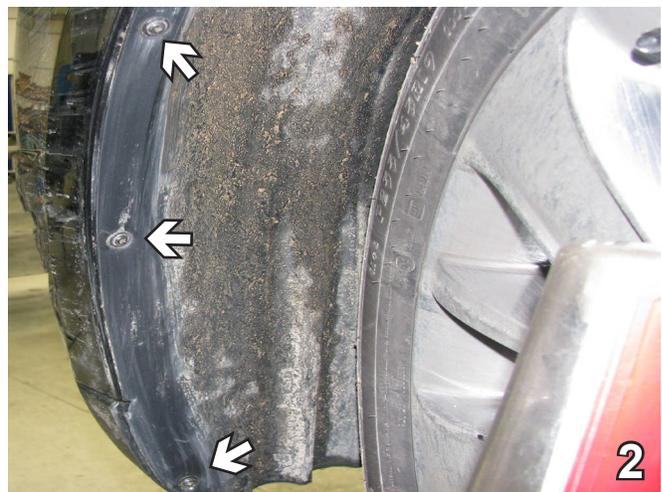
1. Using a 10MM socket, remove two (2) metric bolts from the plastic on top of the fascia. Also remove the one (1) push pin at the top center. Using a Phillips screwdriver, remove the four (4) screws from around the edge (grey arrows). Do this to both sides of the vehicle. Set bolts, push pins and screws aside to be reinstalled later.
