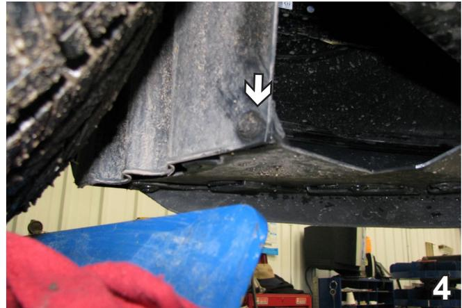
4. Underneath the vehicle in front of the tire, using a 8MM socket remove the bolt in the corner. Do this on both sides. Set the bolts aside to be reinstalled later.
