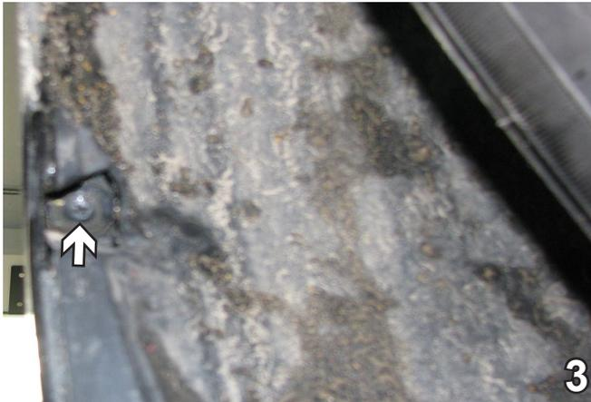
3. In the corner forward of the front tire, remove the push pin. Do this on both sides. Set push pins aside to be reinstalled later.
