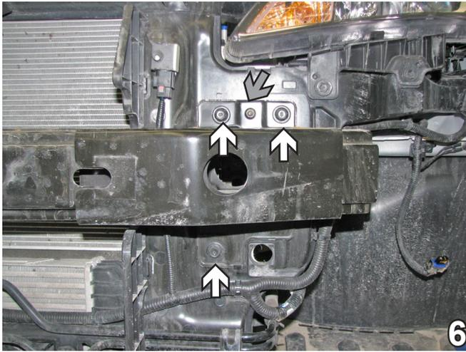
6. Using a 12MM socket, remove one (1) bolt below the bumper and the two (2) outside bolts above the bumper (white arrows). Using a 10MM socket, remove the middle bolt above the bumper (gray arrow). Do this to both sides of the vehicle. Set the bolts and bumper aside to be reinstalled later.
