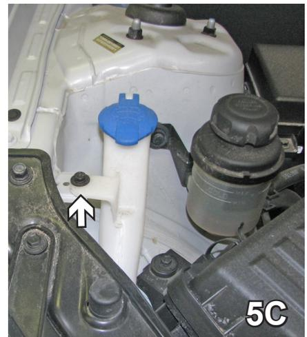
5. On the passenger side, disconnect the hose and electrical connection from the washer reservoir and plug the hose. Using the 10MM socket, remove three metric bolts from the washer reservoir. Remove washer reservoir. Set bolts and reservoir aside to be reinstalled later.
