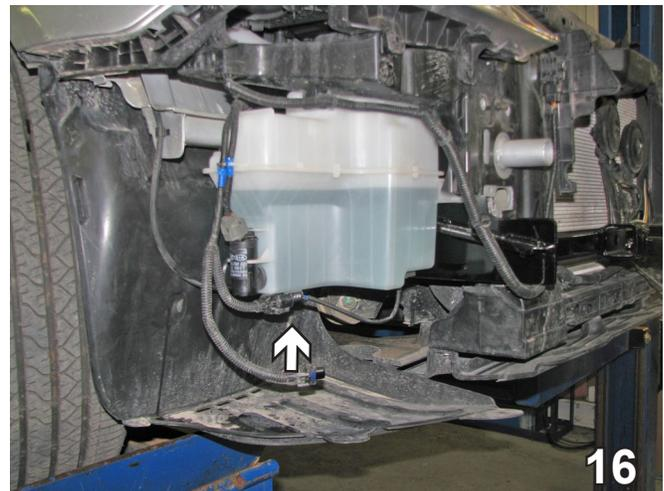
16. On the passenger side, reinstall the washer reservoir using the existing bolts. Reconnect the hose and electrical connection.
