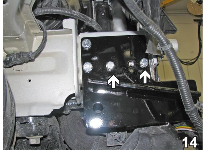
14. Insert 3/8"-16 nut plates through the frame end opening. Align to the lower outside two (2) drilled holes. Install 3/8"-16 x 1-1/4" hex bolts with 3/8" lock washers and tighten. Be sure to use Loctite Red on all bolts. Do this to both sides of the vehicle.
