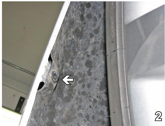
2. Using the 8MM socket, remove one (1) metric bolt from edge of fascia, just inside wheel well. Do this to both sides of the vehicle. Set bolts aside to be reinstalled later.
