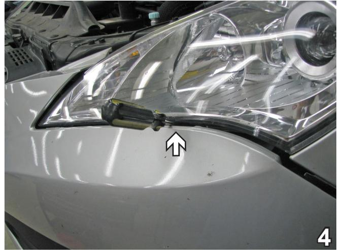
4. Lift up and pull the upper corners of fascia to the side to release from the tabs. Under the headlight use a flat screwdriver to lift up and pull out to unsnap. Do this to both sides of the vehicle. Pull fascia forward to remove. Set fascia aside carefully to be reinstalled later.
