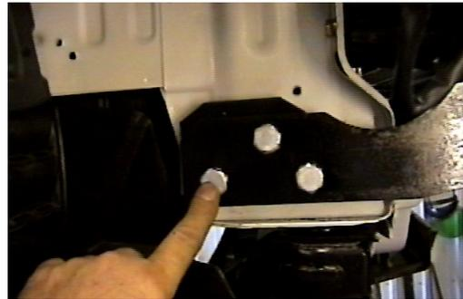
8. Remove the tow brackets with the 17MM socket, both sides. Hold baseplate to align with these holes and install items 3, 4 and 5, both sides. Tighten all bolts. **Note: Use spacer plate, item 3, as needed, apply equally to each side. Be sure and use loctite on all bolts before tightening. Torque all bolts according to torque chart on General Instructions sheet.**
