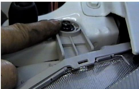
5. Remove two metric bolts with the 6MM socket, pull head light assembly forward, unplug, and set aside, both sides.
