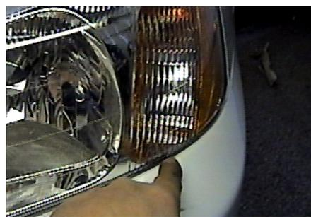
6. Just under head light assemblies is a push pin to remove, both sides. Pull fascia forward and set aside.
