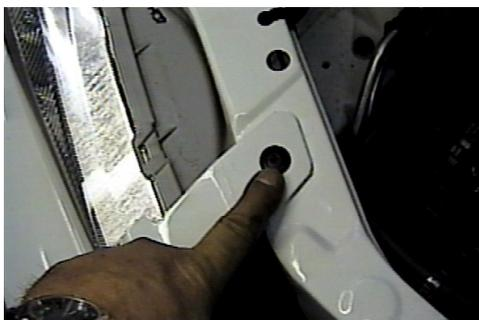
1. Remove the two phillips head push pins from the top side of fascia.
