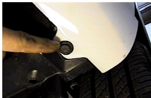
2. There are six phillips head push pins to remove from the bottom side of the fascia.
