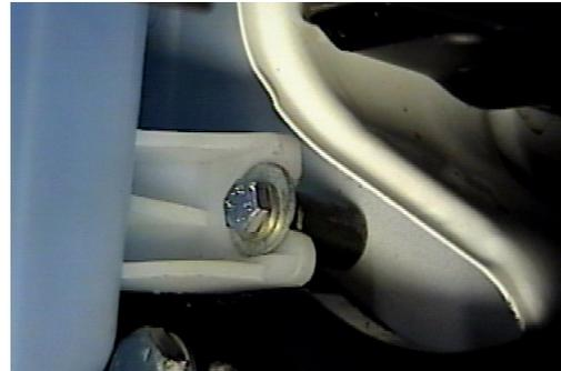
10. To reinstall windshield washer reservoir, it will be necessary to use spacer tube item 14 and item 15 for the front bolt. The upper bolt location will need to be drilled. Reinstall remaining bolts.
