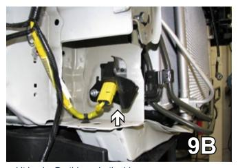
Clamp the air bag sensor bracket with the vice grip and bend it back. Do this on both sides.
