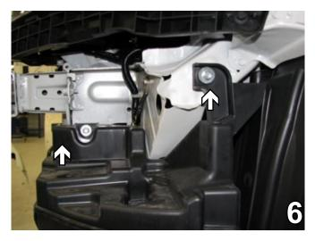
On the driver's side, use a 10MM socket to remove the two bolts holding the air baffle. Don't remove the air baffle just pull it back out of the way. Set the bolts aside to be reinstalled later.
