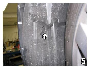
5. On the driver's side, remove the push pin just forward of the front tire in the wheel well. Set the push pin aside to be reinstalled later.
