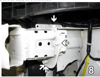
Using a 12MM socket remove the four metric bolts one on each side holding the metal bumper and extension. This is done to both sides. Pull the metal bumper forward and set carefully aside to be reinstalled later.
