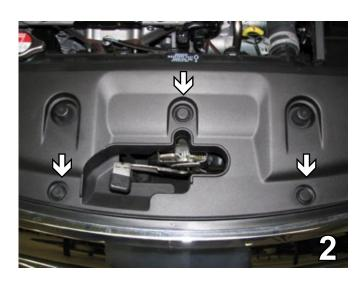
Remove three push pins from the middle in order to remove the radiator cover. Set cover and push pins aside to be reinstalled later.
