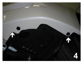
4. Underneath the fascia, remove ten push pins all the way around. Set push pins aside to be reinstalled later.
