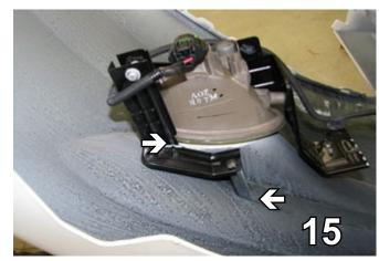
15. On the fog light bracket on the back side of the fascia, cut across the top of the lower bracket and the plastic tab and remove on the driver's side only.
