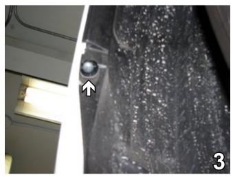
3. In the corner of the fascia, remove the Phillips screw. Do this to both sides of the vehicle. Set screw aside to be reinstalled later.
