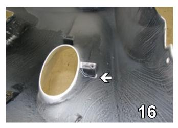
16. Also on the back side of the fascia, cut the tab off on the side of the fog light opening.
