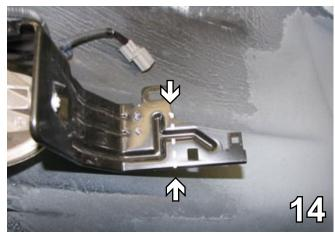
14. Cut the fog light bracket along the slot edge and straight down. Replace the housing to the bracket and reattach back to the fascia. Do this on both sides.
