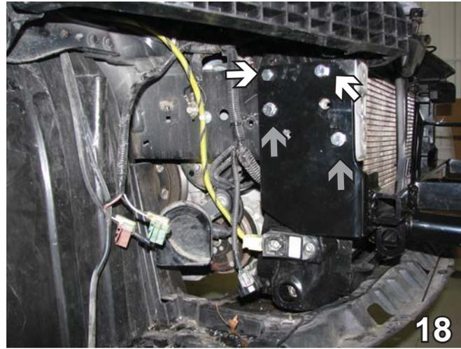
18. On the passenger side upper two holes, install 3/8-16 x 1" hex bolts from the upper frame webbing. Apply loctite and tighten to the 3/8" lock washers and 3/8-16 hex nuts on the outside of baseplate (see white arrows). Insert 3/8-16 nut plate through frame end hole and align to the bottom holes (see grey arrows). Install 3/8-16 x 1 1/2" hex bolt with 3/8" lock washer, apply loctite and tighten to the nut plate.
