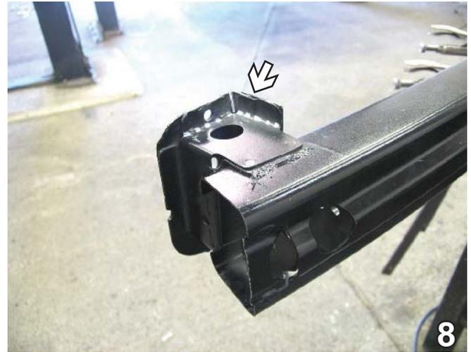
8. With the bottom of the metal bumper face up, mark the back of bumper bracket webbing so it is flush with the bottom edge of bumper. Using the reciprocating saw, cut the marked area to remove lower webbing. Do this to both sides of the vehicle.
