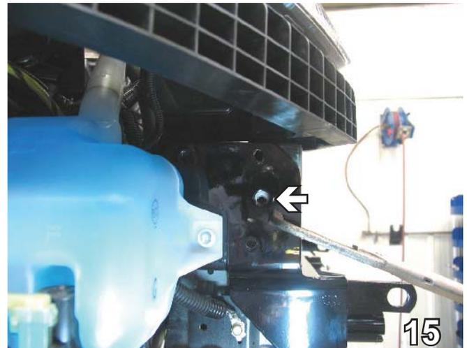
15. Align the baseplate with passenger side existing hole, flush with the top and front edge of the frame rail. Clamp in place using the vice grips. Install the 6mm hex bolt with 6mm lock washer and 1/4" flat washer to the existing hole and tighten with loctite. Using the baseplate as a template, drill the three remaining holes in the passenger's side frame with the 13/32" drill bit.
