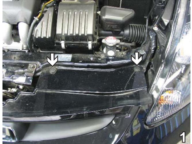
1. On top of the fascia, remove two pushpins between headlights and hood latch. Do this to both sides of the vehicle. Set pushpins aside to be reinstalled later.
