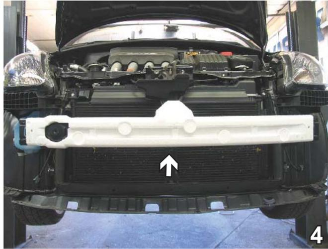
4. Pull styrofoam bumper forward to remove. Set styrofoam bumper aside to be reinstalled later.
