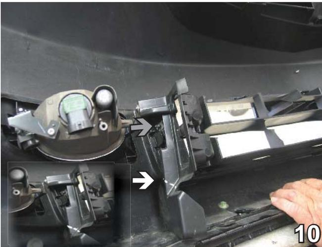
10. Lay fascia face down on a soft, non-marring surface. Using the utility knife, trim horizontally across the fascia support molding next to the grille (see white arrow). Remove one Phillips screw from the fascia support (see grey arrow). Remove upper portion of fascia support. Do this to both sides of the vehicle.
