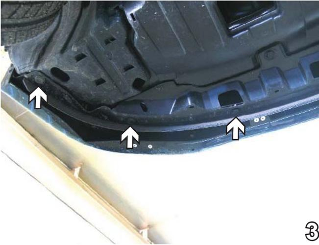
3. Remove eight pushpins from bottom of fascia (three each side and two in the center). Pull upper corners of fascia to the side to release tabs. Do this to both sides of the vehicle. Pull fascia forward to remove. Set pushpins and fascia aside carefully to be reinstalled later.
