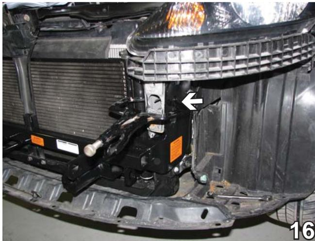
16. On the driver's side, use the baseplate as a template to drill the front bottom hole in the frame with the 13/32" drill bit. Insert 3/8-16 nut plate through frame end hole and align to the drilled hole. Install 3/8-16 x 1 1/2" hex bolt with 3/8" lock washer and tighten with loctite to the nut plate.
