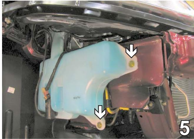
5. Using a 10MM socket remove two metric bolts from the washer reservoir. Do not remove the reservoir.
