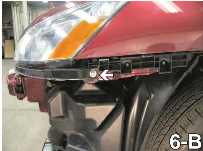
6. Using the 10MM socket, remove the four metric bolts from the top side of the head light assembly, indicated by the white arrows in the photo 6-A. Remove one metric bolt on the side, indicated by the grey arrow in the photo 6-B. Pull assembly forward disconnect electrical connections. This is done to both sides of the vehicle, the driver's side is shown. Set headlights aside to be reinstalled later.
