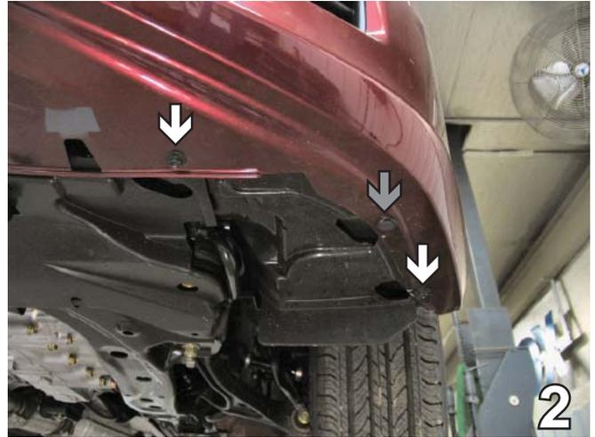
2. Using 10MM socket remove two metric bolts from the lower edge of the fascia just forward of the front tire, as indicated by the white arrows in the photo above. Remove one push pin indicated by the grey arrow in the photo above. Do this to both sides of the vehicle, the driver's side is shown.
