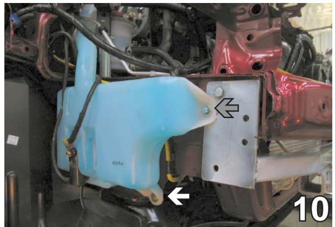
10. Reinstall lower washer reservoir bolt with existing bolt, indicated by the white arrow in the photo above. Use a 6MM-1 x 30MM hex bolt, 1/4" lock washer and 1/4" flat washer for the front bolt's location, indicated by the grey arrow in the photo above.
