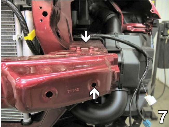
7. Using a 12mm socket remove two metric bolts from the top of the metal bumper and on the bottom. Pull the metal bumper forward and set carefully aside. This is done to both sides, the driver's side is shown.
