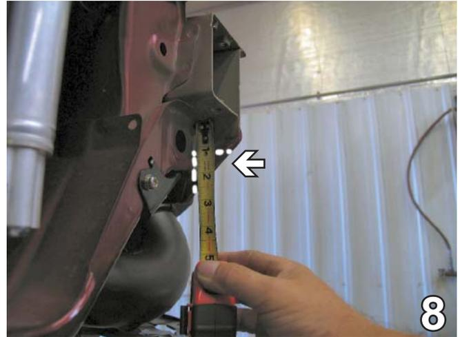
8. Measure 1 1/4" down from the bottom of the frame rail. Make a horizontal mark on the webbing back to cross member and down. Using a reciprocating saw remove this portion of the frame. Do this on both sides, the driver's side is shown.
