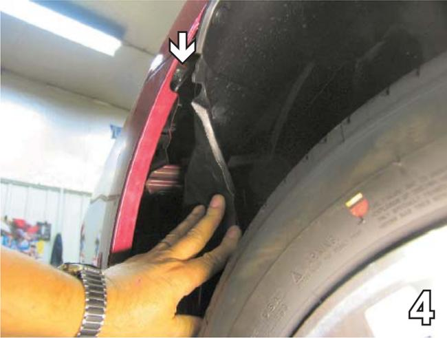
4. Just forward of the front tire on fascia's corner, remove on Phillips head screw with the Phillips screw driver. Do this to both sides of the vehicle, the driver's side is shown. Pull the fascia corner out to the side of the vehicle and then forward to release, set fascia aside carefully.
