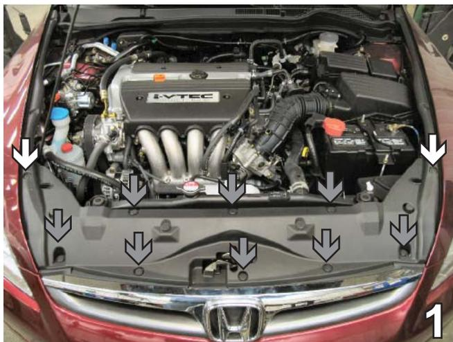
1. Remove the Phillips head push pins, indicated by the white arrows in the photo above. Also remove five push pins from the front edge just above the grill and three push pins from the back edge of black plastic cover on the top side of the fascia. These are indicated by the grey arrows in the photo above lift cover and set aside to be reinstalled later.
