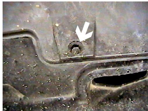
6. Remove one metric bolt from lower edge of fascia with the 10MM socket, both sides, pull fascia forward and set aside.
