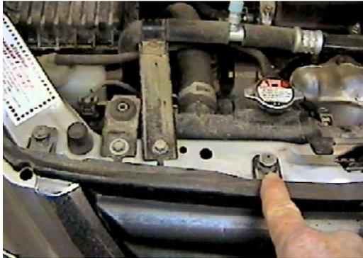
1. Remove the four phillips screws from top edge of upper grill between headlights, using the phillips screw driver.
