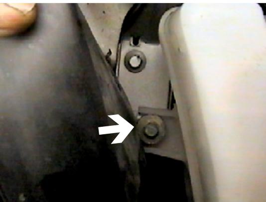
11. Using the 10MM socket, remove one metric bolt from air baffle on passenger's side.
