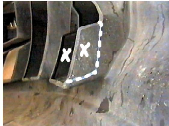
20. Using a utility knife, cut and remove the marked pieces from the back side of fascia, both sides.
