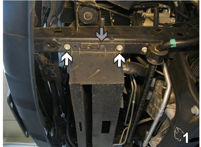
1. Remove belly pan from under the vehicle. Using a 13MM socket, remove two bolts and also one push pin (gray arrow) with a flat screwdriver. Do this to both sides. Set aside for later reinstallation.
