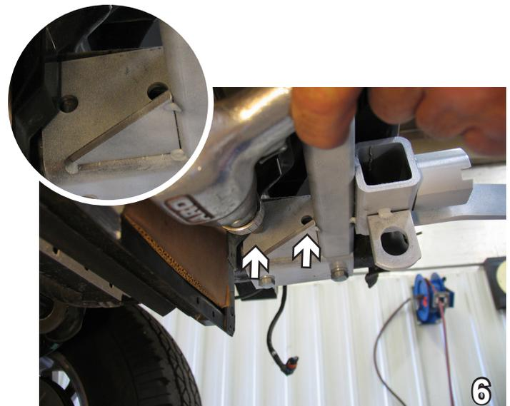
6. While using the baseplate as a template, drill the two holes located inside of the baseplate closest to the radiator. Drill with a 17/32" drill bit. Do this to both sides. Install a 1/2 x 1 1/2" hex bolt and 1/2" lock washer to each of the drilled holes into nut plate.
