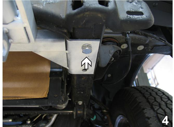
4. Install the baseplate by first installing 1/2 x 1 1/2" lock washer with nut plate in first hole that lines up with existing hole. If hole in frame end is not quite big enough to install nut plate, use hammer to widen opening. Do this to both sides.
