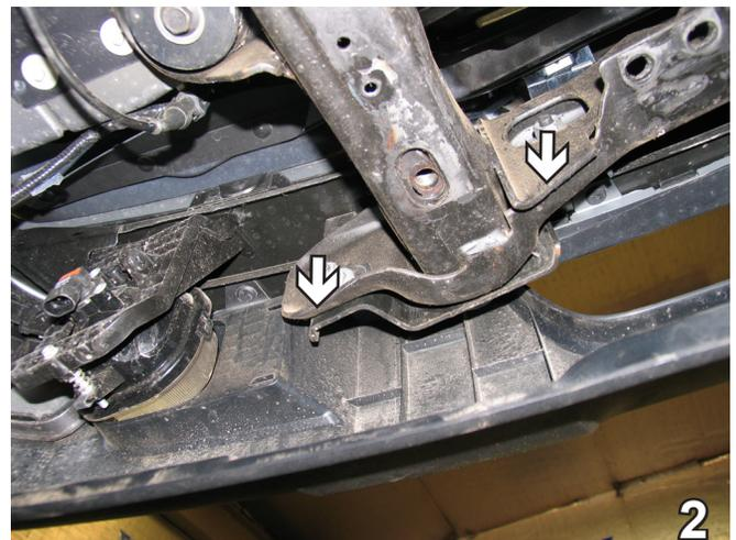
2. To remove front bumper, go underneath vehicle on backside of bumper to remove two hex nuts with a 18MM socket. Do this to both sides. Place hex nuts and bumper aside for later reinstallation. Unplug the foglights if available.
