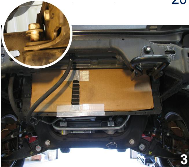
3. Place a piece of cardboard over radiator to keep from bending fins. While using a 15MM socket, remove three bolts behind tow hooks (inset circle). Remove tow hooks. Do to both sides. Tow hooks will not be reinstalled.
