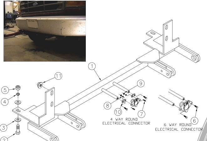
**IMPORTANT:** Use only genuine factory replacement parts on your Base Plate. Do not substitute homemade or nontypical parts. If a bolt is lost or in need of replacement, for your safety and the preservation of your Base Plate, be sure to use a replacement bolt of the same grade (Usually Grade 5, refer to parts list). Repair parts may be ordered through your nearest **Blue Ox** dealer or distributor.
