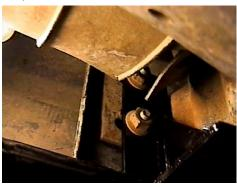
3. Align item 1 with the existing bolts on the back side of the metal bumper and snug existing nuts in place. Be sure and use loctite on all bolts before tightening. Tighten all bolts according to torque chart in the General Instruction Sheet.
