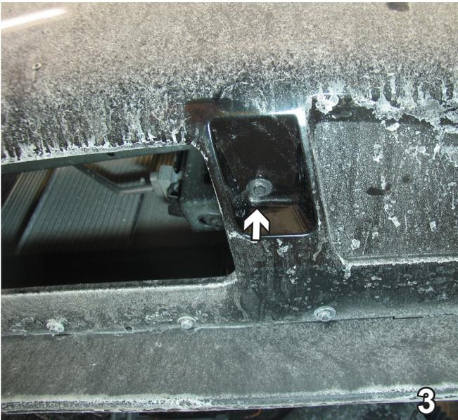
3. Using a 10MM socket, remove one metric bolt located on the side of the opening in the fascia. Set bolt aside to be reinstalled later. Do this to both sides of the vehicle.
