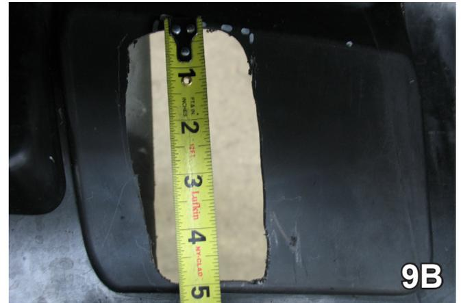
9. Using a hack saw knife, mark and trim out opening in the fascia for the attachment tabs, using the photos above as a template. Do this to both sides of the vehicle. Models that have tow hooks will not need to cut out opening in fascia.
