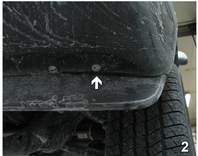
2. Using a 10MM socket, remove one metric bolt from the front of the fascia. Set bolt aside to be reinstalled later. Do this to both sides of the vehicle.
