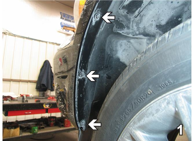
1. Using a 10MM socket, remove three metric bolts just forward the front tire, on the wheel well. Once bolts are removed from the wheel well, pull plastic back and remove two metric bolts with a 10MM socket. Set bolts aside to be reinstalled later. Do this to both sides of the vehicle.
