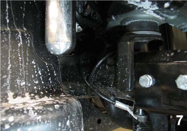
7. Attach permanent baseplate safety cables to the convenience link on the baseplate. The photo above shows recommended installation of the cables to frame of vehicle. If vehicle has additional options (not shown above) which interfere with mounting permanent baseplate safety cables, secure the cables to a solid piece of the vehicle frame as described in instructions included with the permanent baseplate safety cables.
