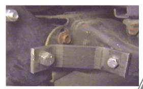
6. Install item 3 using items 9, 10,11, and 12 to bumper brackets existing hole, and tighten. Using the brace as a template, drill 13/32" hole and fasten with items 5, 6, 7, and 8. both sides. Be sure and use loctite on all bolts before tightening.
