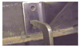
5. Using a clamp, hold lower support to cross member. Drill these holes with the 13/32" drill bit, both sides. Insert item 5 thru baseplate and cross member into item 4. Tighten items 7 and 8, according to drawing on last page.
