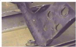
3. To remove bumper bracket, use the 18MM socket. It will be necessary to remove bottom carriage bolt with a pry bar. Reinstall bumper brackets to vehicle and center baseplate on brackets, mark and drill holes with the 13/32" drill bit, both sides.
