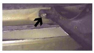
7. Install metal bumpers upper carriage bolts and nuts to bracket using the 18MM socket, do **not** tighten.
