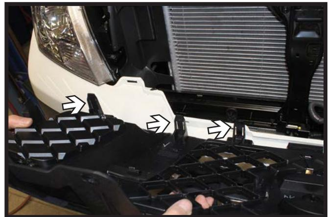
2. **2011 & Older Models:** To remove the grille, turn the two (2) square pins (inset). Then reach in and push up on the two (2) clips. Do this on both sides and remove the grille.
