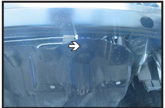
9. Using the 10MM socket, remove the two (2) bolts from the belly pan that bolt into the bottom of the metal bumper.
