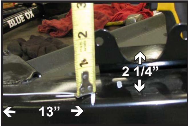
17. Set the metal bumper on a bench, clamp the electrical bracket to the back of the driver's side with the vise grip. The bracket should measure 13" from the driver's end of the metal bumper and 2 1/4" from the top edge of the bumper to the top hole location. Attach the bracket with the two (2) #10-16 self drilling screws using the 5/16" nut driver. Reinstall the metal bumper with the existing bolts. Reinstall the fascia.
