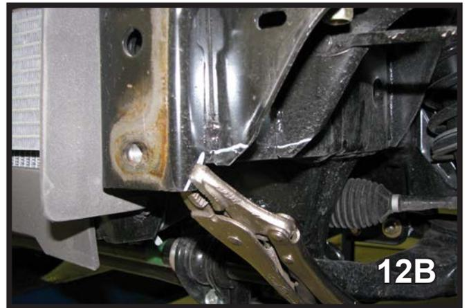
12. Using the vise grip bend the frame support, approximately 1/2" up from the bottom, back and fourth until it snaps off on both the front and back supports. Do this on both sides. (14A)
