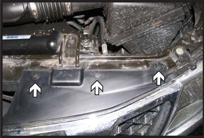
1. Remove three (3) push pins from the top of the grille. Do this on both sides.
