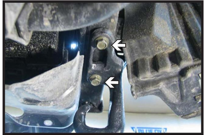
11. Remove the two (2) bolts from the tow hook on the passenger's side only using a 17MM socket. **The tow hook will NOT be reinstalled.**
