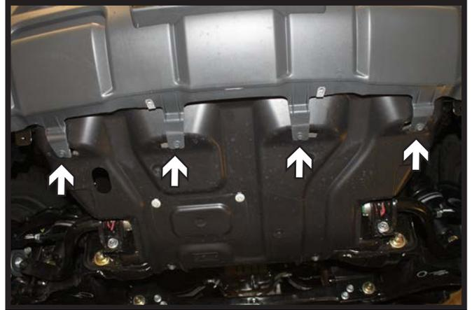
6. Using a 10MM socket, remove the four (4) screws from the underside of the fascia.
