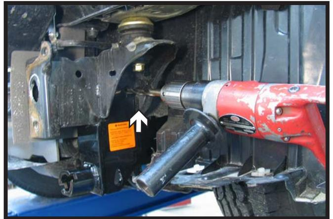
14. Using the baseplate as a template, drill a hole into the side of the frame rail with the 17/32" drill bit. Do this on both sides.
