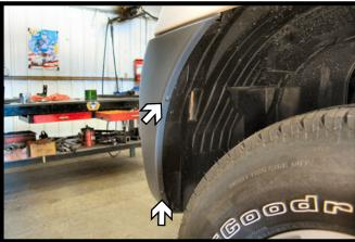
4. Using a Phillips screwdriver, remove the two (2) screws from the wheel well. Do this on both sides of the vehicle.
