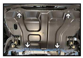
10. Remove the four (4) screws from the belly pan and set the pan aside.
