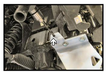
13. Using a 17/32" drill bit, drill the hole in the side of the baseplate thru the frame. Install a 1/2"-13 x 1-1/2" bolt with 1/2" lock washer into the hole and a 1/2" nut plate on the inside of the frame. Do this on both sides of the vehicle. Fully tighten hardware.
