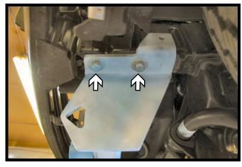
12. Position the baseplate onto the vehicle. Install 12MM-1.25 x 45MM bolts with 12MM lock and 1/2" flat washers into the existing holes. Do this on both sides of the vehicle. Fully tighten hardware.
