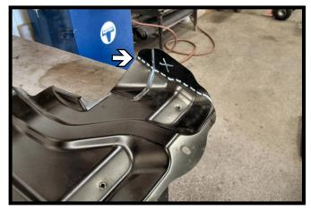
14. Using a reciprocating saw, trim the outer flange off the belly pan as shown. Do this on both side of the pan.
