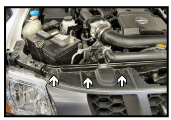
1. Remove the six (6) push pins from the top edge of the grille. There are three (3) on each side of the vehicle.
