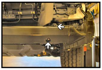
9. Using a 17MM socket, remove the four (4) bolts from the bumper. There are two (2) on each side. Set the bumper aside.
