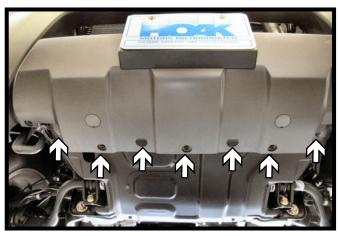
6. Using a 10MM socket, remove the seven (7) screws from the underside of the fascia.
