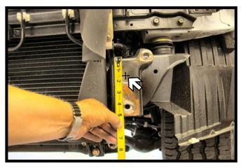
11. Using a 1-1/4" hole saw, drill an access hole 1-3/4" down from the top of the frame and centered side to side. Do this on both sides of the vehicle.
