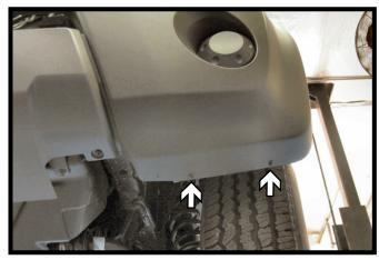
5. Using a Phillips screwdriver, remove the four (4) screws from the underside of the fascia. There are two (2) on each side.
