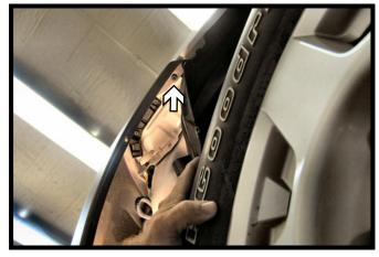
7. Pull back the wheel well liner, remove the screw from the top edge of the fascia. Do this on both sides of the vehicle. Pull the fascia forwards disconnecting any electrical connections and set fascia aside.
