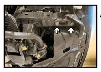
3. Using a 17MM socket, remove the two (2) bolts from the tow hook bracket. Do this on both sides of the vehicle. Tow Hooks will not be re-installed.
