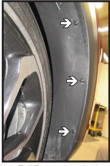
2. Using a T15 Torx, remove the three (3) bolts from the wheel well edge. Do this on both sides of the vehicle.
