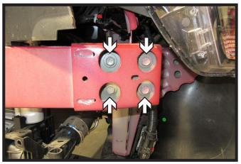
Using a 15MM socket, remove the four
