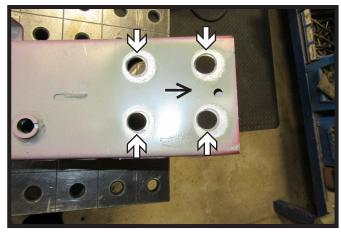
14. Slightly slot the four (4) holes in the bumper towards the outside. Do this on both sides of the bumper.
