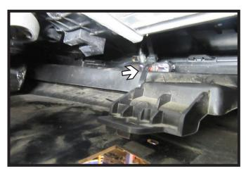
28. Start reinstalling the fascia. Before reinstalling bottom bolts, relocate and secure temperature sensor using provided 9" zip tie.
