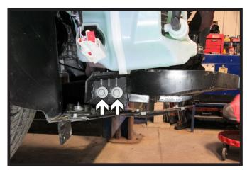
11. Using a 13MM socket, remove the two (2) bolts from plastic piece below the windshield washer reservoir. Do this on both sides of the vehicle. Remove piece and set aside to be reinstalled later.
