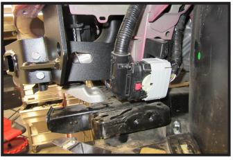
22. Reattach electrical loom to frame on the driver side of the vehicle.
