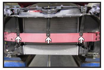
13. Using a 10MM socket, remove the three (3) bolts from the bumper support brackets. Remove bumper and set aside to be reinstalled later.
