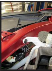
12. Using a 10MM socket, remove the two (2) nuts (white), one (1) bolt (gray), and one (1) push pin (black) from the windshield washer fluid reservoir on the passenger side of the vehicle. Disconnect and plug all lines. Remove reservoir and set aside to be reinstalled later.
