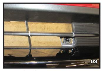
25. Unclip temperature sensor from the bracket on the back of the fascia. Then using a reciprocating saw trim each side of the fascia as shown to allow room for the baseplate and convenience link.
