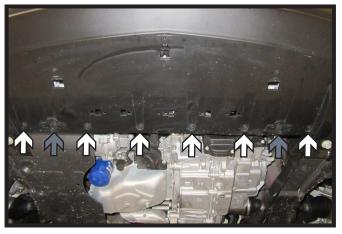
Using a 7MM socket, remove the six (6) bolts (white) from the bottom of the fascia. Then remove the two (2) push pins (gray).
