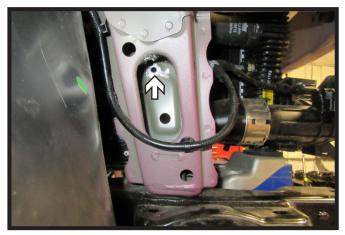
19. Using a 1/4" drill bit, create starter hole in frame on the passenger side of the vehicle. Then using a 1/2" drill bit, drill out top hole in frame.
