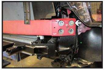
16. Slide the baseplate onto the vehicle between the frame and the bumper. Start one (1) existing 10MM bolt in the top outer hole. Do this on both sides of the vehicle. Ensure the holes on the bumper line up with the baseplate and tighten the six (6) bolts on the support brackets.
