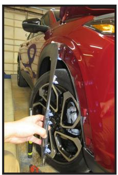
3. Pull back the wheel well trim, releasing the nine (9) push pins, past the fascia joint.
