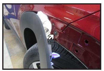
4. Using a 7MM socket, remove the one (1) bolt from the fascia joint. Do this on both sides of the vehicle.
