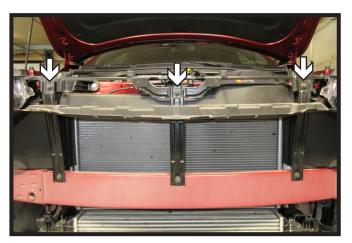
15. Reattach bumper to support brackets, leave loose. Then using a 10MM socket, loosen the top three (3) support bracket bolts.
