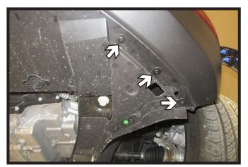
5. Using a T15 Torx, remove the three (3) bolts from the bottom of the fascia. Do this on both sides of the vehicle.
