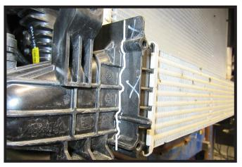
10. Using a reciprocating saw, trim the plastic as shown for baseplate clearance. Do this on both sides of the vehicle.
