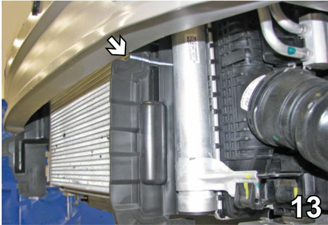
13. Using the utility knife, cut the plastic air dam along the top even with the bottom of the bumper and remove lower section. Do this on both sides.
