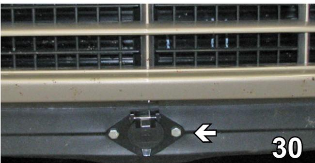
30. Possible location to mount the 4 or 6 pin electrical coupler on the fascia's lower air dam.
