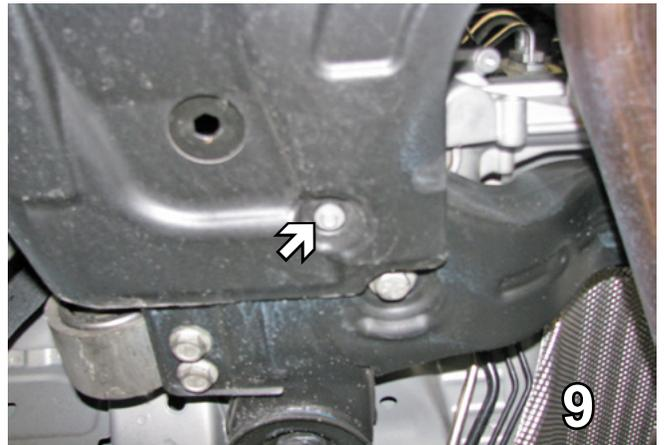
9. Using an 8MM socket, remove one (1) more metric bolt toward the back of the belly pan. Do this on both sides. Set bolts aside to be reinstalled later.
