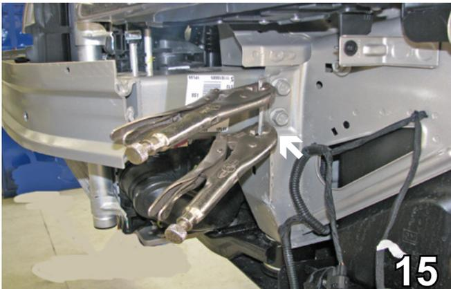
15. Using vice grips, bend the frame webbing over and flatten with a hammer. Do this on both sides.
