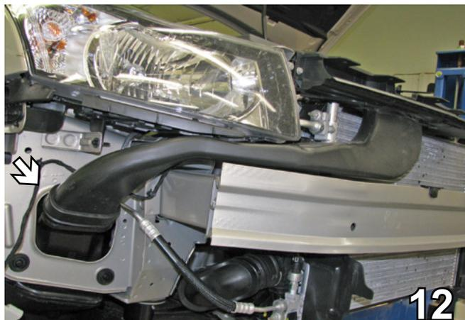
12. On the passenger side below the headlight, detach the air intake tube from the bottom section of the tube. Set aside to be reinstalled later.
