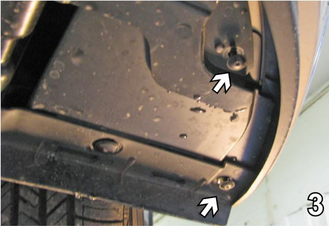
3. Remove the two (2) bolts from underneath the fascia, just forward of front tires with the T20 Torx, both sides. Set the bolts aside to be reinstalled later.
