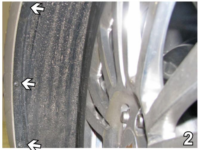
2. Just forward of front tire, on the edge of the wheel well, are three (3) bolts to remove with the T20 Torx, both sides. Set bolts aside to be reinstalled later.
