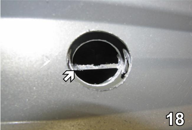
18. Inside the 1-1/2" drilled hole is a cross piece, which may need to be bent vertically with a pry bar in order to insert 3/8" nut plate. Do this on both sides.
