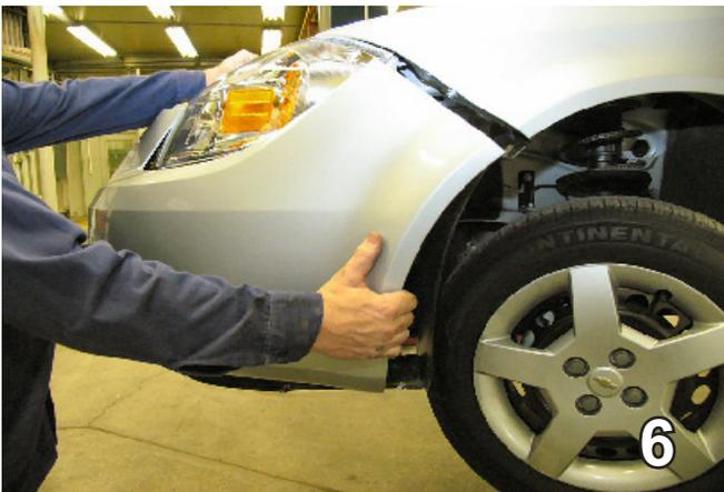
6. Lift up the black plastic just above radiator (step 1), pull fascia's corner out to the side, pull fascia forward both sides, unplug all electrical components if necessary and set fascia aside carefully.
