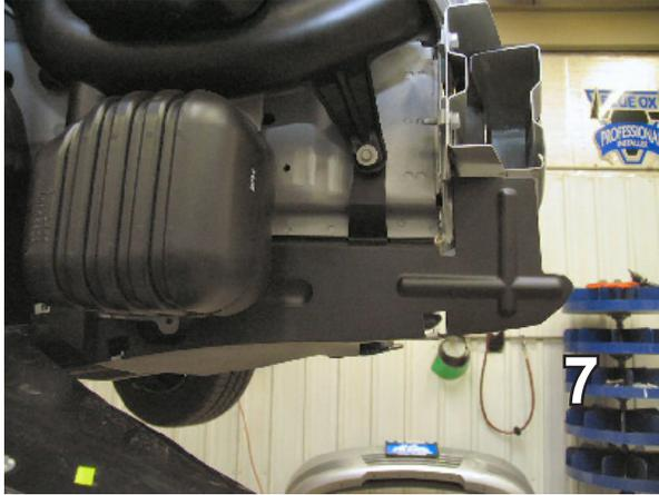
7. Remove the metric bolt from the air ram intake tube on the passenger's side with the 10MM socket.
