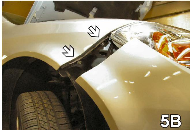
5. Remove the lower metric bolt just forward of the front tire (left photo), on fascia's upper corner, using the 10MM socket, both sides. Loosen the top and bottom remaining metric bolts to release fascia's corner, with the 10MM socket, both sides.
