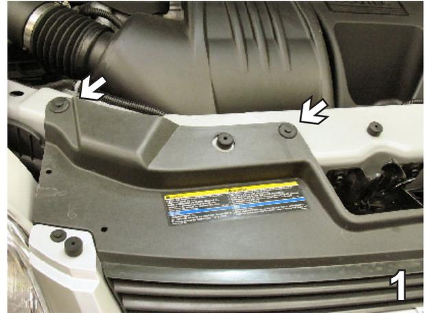
1. Remove the two push pins from the black plastic cover just above the radiator, both sides.
