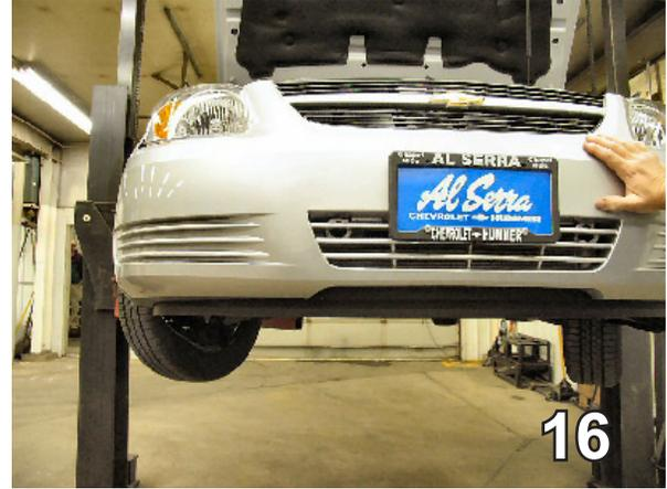
16. Hold fascia as close to its original position as possible, mark and cut the top style of the lower grill opening, on both sides of the attachment tab receivers to allow tabs to come through. Reinstall fascia. **Be sure all electrical components are plugged in properly.**
