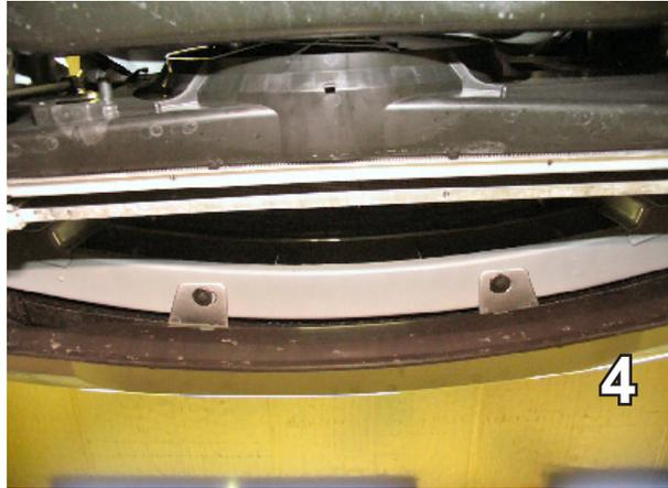
4. Remove the two push pins from the fascia tabs, just below metal bumper, behind fascia.
