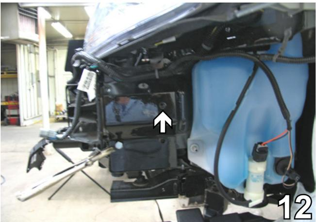
12. Align the baseplate on the driver's side so the upper back hole aligns with the existing horn bracket hole and clamp in place with vise grips. Reinstall the horn bracket with the existing bolt. Using the baseplate as a template, drill the remaining three holes into the frame rail on the driver's side with the 13/32" drill bit.
