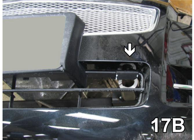
17. Hold fascia as close to the original location as possible and mark area to be removed. Trim 2 1/2" of the upper rib off to give room for baseplate. Do this on both sides of the vehicle. Some models may need more trimming (gray arrows) check the fascia fit.
