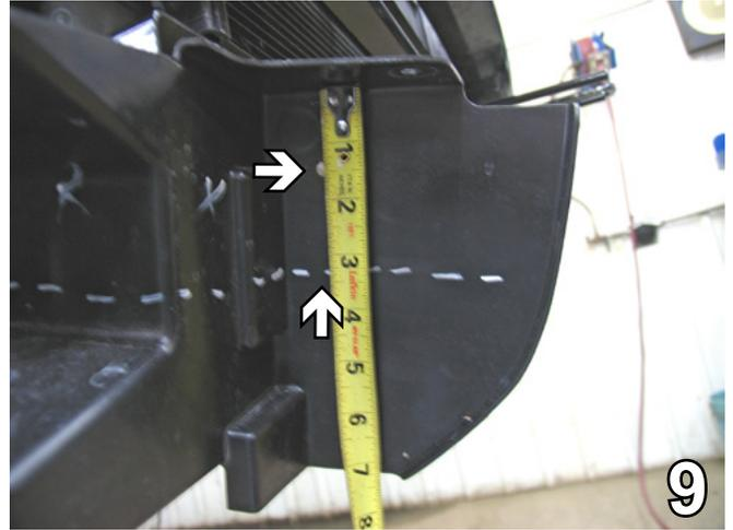
9. **2008-09 Models:** Mark the passenger's side of the air dam straight down 3 inches where the hole is and around the contour of the air dam mold.
