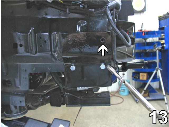
13. Align the baseplate on the passenger's side so the upper back hole aligns with the existing air intake value hole into which a push pin will be inserted. Using the baseplate as a template, drill the three remaining holes into the frame rail on the passenger's side with the 13/32" drill bit.
