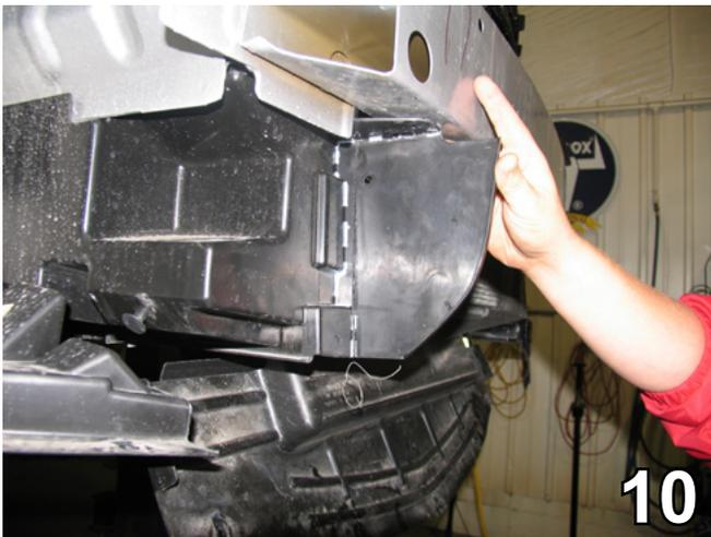
10. **2010-11 Models:** Mark the air dam straight across the top and straight down the side, as shown, and trim.
