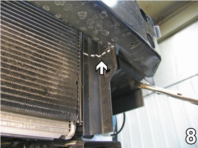
8. Using the utility knife, trim the piece of plastic right next to the radiator flush with the bottom of the bumper. Discard the lower portion. Do this on both sides.
