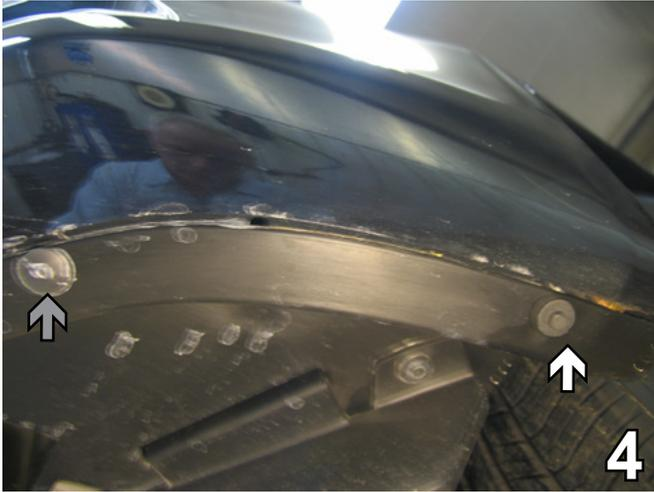
4. Using the 7MM socket, remove nine metric bolts from underneath corner of the front fascia, forward of the front tire, as indicated by the white arrow in the photo above. Remove two pushpins, as indicated by the grey arrow in the photo above. Do this around the vehicle. Remove fascia by pulling it out to the side and forward a little bit. Set fascia, bolts and pushpins aside carefully to reinstall later.
