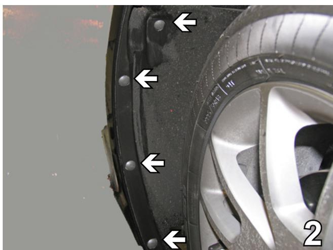
2. Just forward of the front tire, on the edge of the wheel well cover, remove four pushpins. Do this to both sides of the vehicle. Set pushpins aside to reinstall later.
