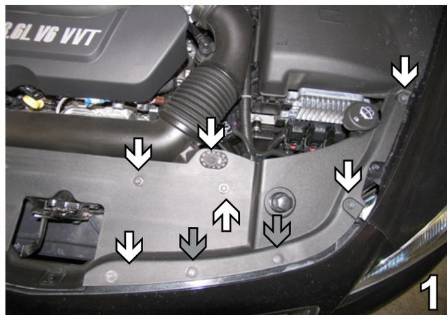
1. Using the 10MM socket, remove six bolts from the black plastic cover on the driver's top side of the fascia (white arrows). Using the Phillips screwdriver, remove the two Phillips pushpins (gray arrows). On the passenger side remove five bolts and two pushpins. Set bolts, pushpins and plastic cover aside to reinstall later.
