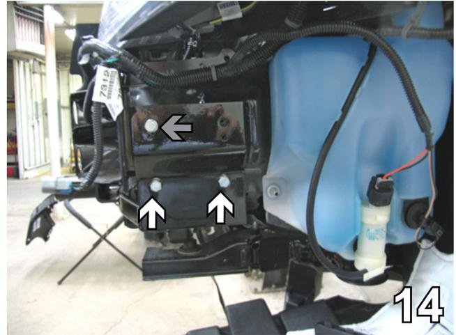
14. Insert two 3/8-16 x 1" hex bolts, 3/8-16 hex nuts and 3/8 lock washers into the bottom two holes. Use Loctite Red on all the bolts. Guide a 1" nut plate up through the opening in the bottom of the frame rail and align it with the upper front bolt hole. Install the 3/8-16 x 1 1/2" hex bolt and the 3/8" lock washer to the 1" nut plate, as indicated by the grey arrow in the photo above. Do the same on the passenger side.
