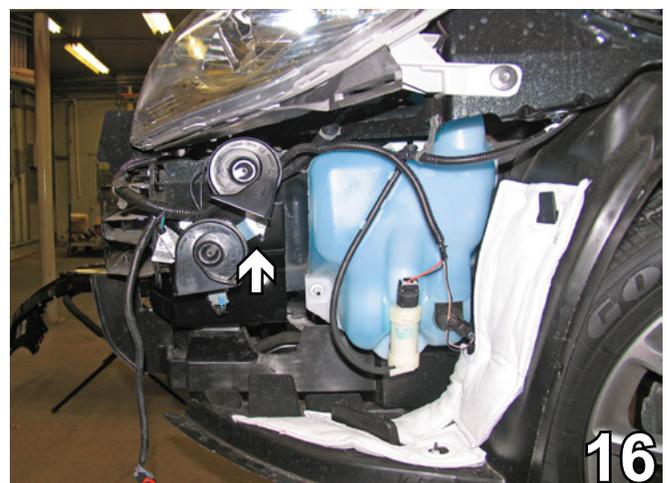
16. Reinstall the horn on the driver's side.
