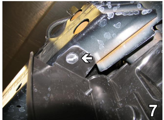
7. Remove pushpin from the bottom of the bumper. Do this on both sides. Set pushpin aside to reinstall later.
