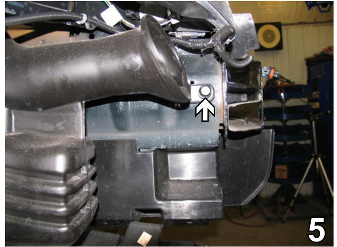
5. Remove pushpin from the passenger's side air baffle. Set air baffle and pushpin aside to reinstall later.
