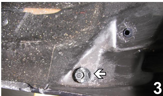
3. Also just forward of the front tire, on the edge of the wheel well cover, using the 10MM socket, remove the bolt. Do this to both sides of the vehicle. Set bolts aside to reinstall later.
