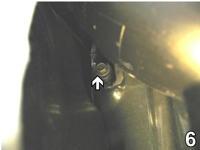
6. Using the 10MM socket, remove one metric bolt from the back side of the air baffle. Set air baffle and bolt aside to reinstall later.
