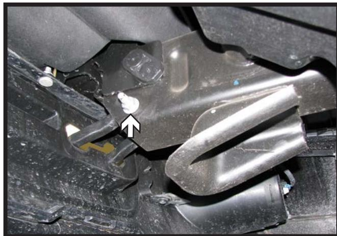
2. Using a 18MM socket, remove one nut from the outside edge of the frame rail. Pull the tow hook forward and remove it. Do this to both sides of the vehicle. The factory tow hooks will not be reinstalled.
