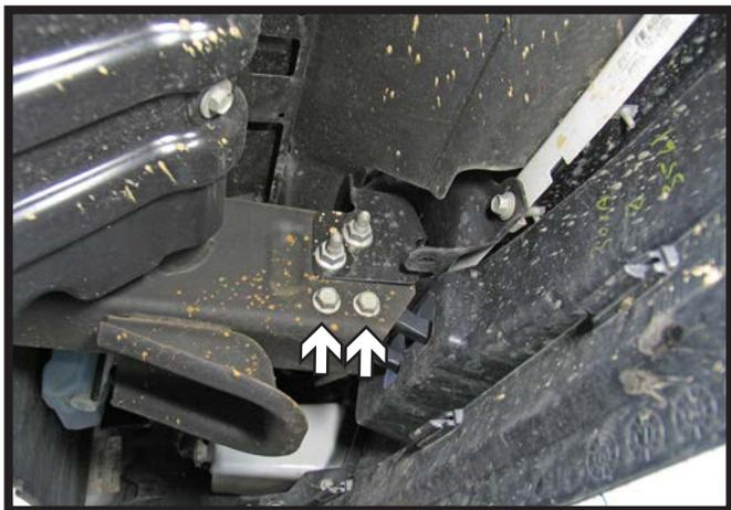
1. Using a 18MM socket, remove two (2) bolts from the inside edge of the frame rail. Do this to both sides of the vehicle. This hardware will not be reinstalled.
