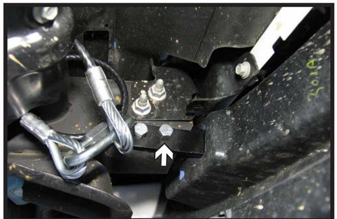
8. Slide the baseplate into frame end to align with the front tow hook hole on the outside of the frame rail. Insert straight portion of the convenience link thru the tow hook opening and align it with the existing holes of the frame. Insert a 1/2"-13 x 5" bolt thru the frame with a 1/2" lock washer and 1/2" lock nut on the other side and tighten down. Do this to both sides of the vehicle.
