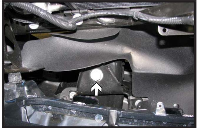
6. Remove the bolt on top of frame end, just below plastic removed in Step 4 with a 21MM socket. Reinstall the bolt with four (4) 1/2" flat washers. Do this to both sides, one side at a time.
